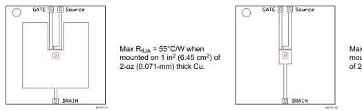
Max  $R_{\theta JA}$  = 160°C/W when mounted on a minimum pad area of 2-oz (0.071-mm) thick Cu.
