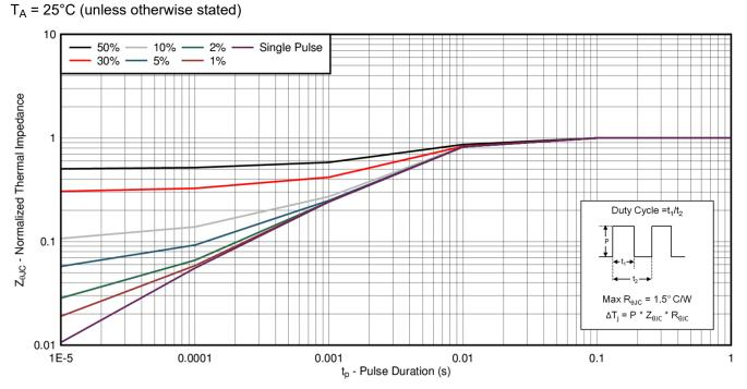
Figure 5-1. Transient Thermal Impedance
