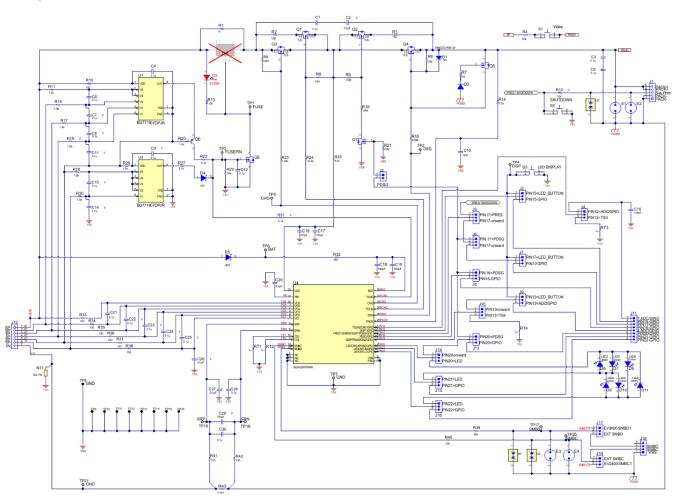
Figure 9-1. BQ40Z80EVM Gauge and Protector Schematic
