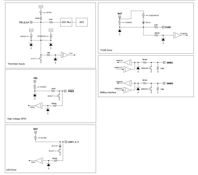
Figure 6-3. Pin Equivalent Diagram 2
