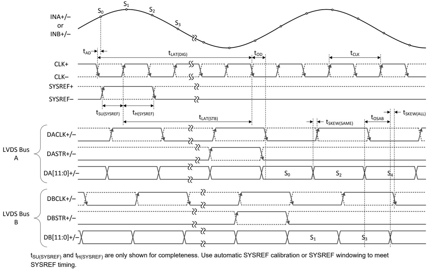
**Figure 5-4. Single-Channel, 2-Bus, Staggered-Mode Timing (LDEMUX = 0, DES\_EN = 1, LALIGNED = 0)**
