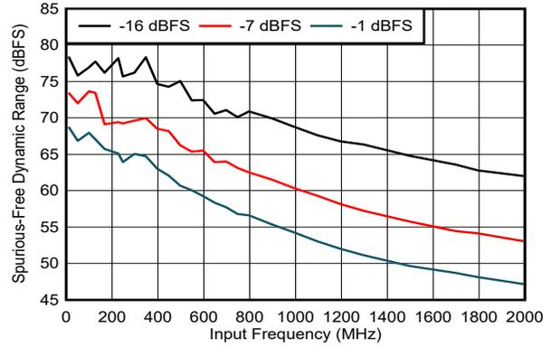
DES\_EN = 1,  $f_S = 2000\text{MHz}$ , FG calibration
