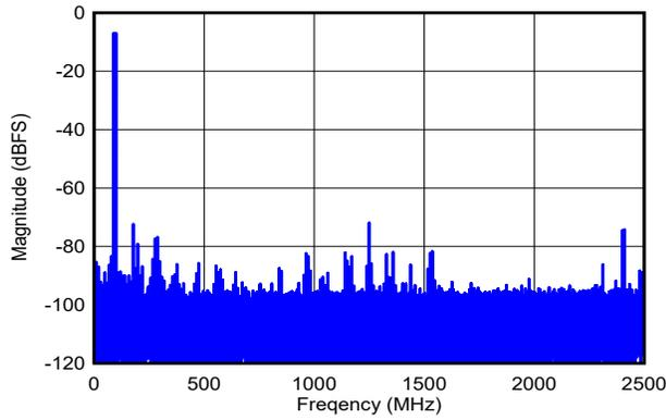
DES\_EN = 1,  $f_S = 5000\text{MHz}$ , FG calibration,  $f_1 = 89\text{MHz}$ ,  $f_2 = 99\text{MHz}$ ,  $A_{IN} = -7\text{dBFS}$  per tone, SFDR =  $-72\text{dBFS}$ , IMD3 =  $-86\text{dBFS}$ , IMD2 =  $-86\text{dBFS}$
