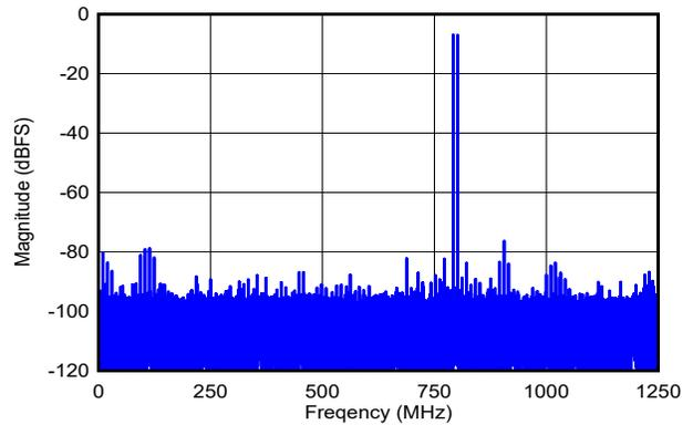
DES\_EN = 0,  $f_S = 2500\text{MHz}$ , FG calibration,  $f_1 = 792\text{MHz}$ ,  $f_2 = 802\text{MHz}$ ,  $A_{IN} = -7\text{dBFS}$  per tone, SFDR =  $-76\text{dBFS}$ , IMD3 =  $-91\text{dBFS}$ , IMD2 =  $-78\text{dBFS}$
