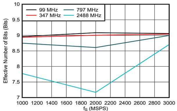
DES\_EN = 1,  $f_S = 3000\text{MHz}$ , FG calibration
