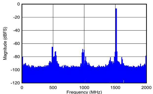
DES\_EN = 1,  $f_S = 4000\text{MHz}$ , FG calibration,  $f_1 = 2483\text{MHz}$ ,  $f_2 = 2493\text{MHz}$ ,  $A_{IN} = -7\text{dBFS}$  per tone, SFDR =  $-65\text{dBFS}$ , IMD3 =  $-73\text{dBFS}$ , IMD2 =  $-73\text{dBFS}$
