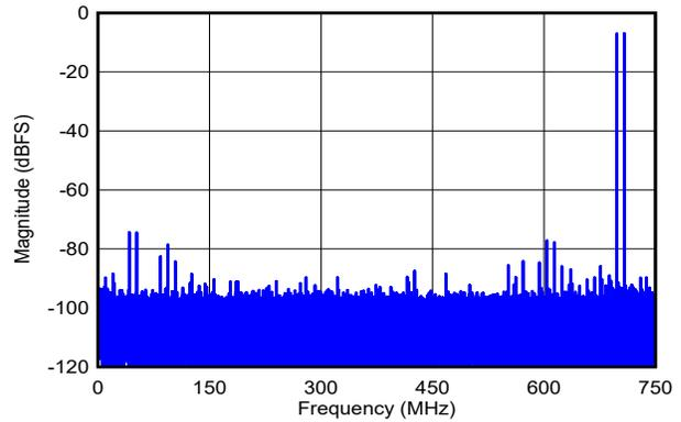
DES\_EN = 0,  $f_S = 1500\text{MHz}$ , FG calibration,  $f_1 = 792\text{MHz}$ ,  $f_2 = 802\text{MHz}$ ,  $A_{IN} = -7\text{dBFS}$  per tone, SFDR =  $-74\text{dBFS}$ , IMD3 =  $-90\text{dBFS}$ , IMD2 =  $-82\text{dBFS}$
