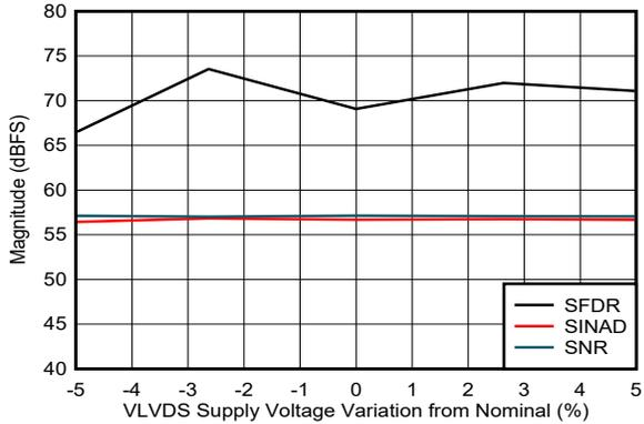
DES\_EN = 0,  $f_S = 1500\text{MHz}$ ,  $F_{IN} = 347\text{MHz}$ ,  $A_{IN} = -1\text{dBFS}$
