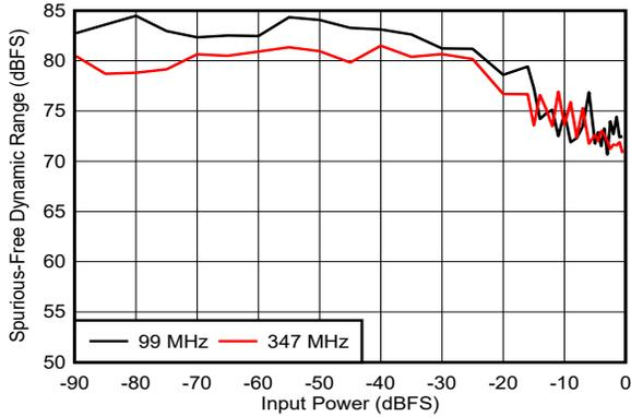
DES\_EN = 0,  $f_S = 500\text{MHz}$ , FG calibration
