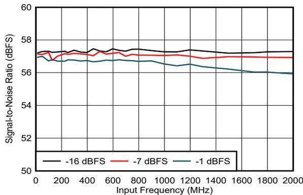
DES\_EN = 0,  $f_S = 2000\text{MHz}$ , FG calibration
