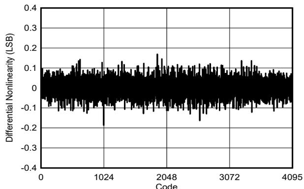
DES\_EN = 1,  $f_S = 5000\text{MHz}$ , FG calibration,  $F_{IN} = 99\text{MHz}$
