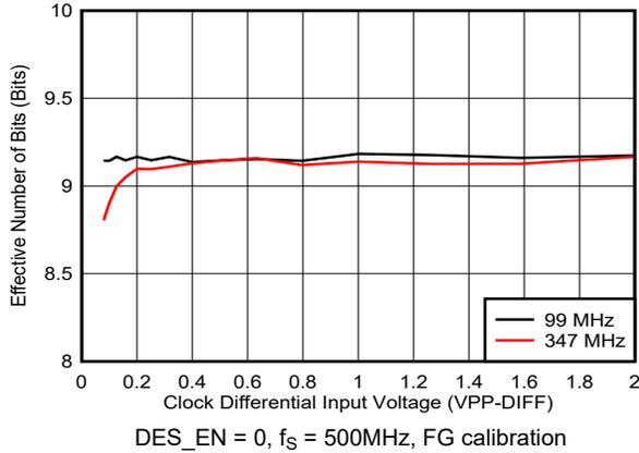
**Figure 5-34. ENOB vs Clock Amplitude**
