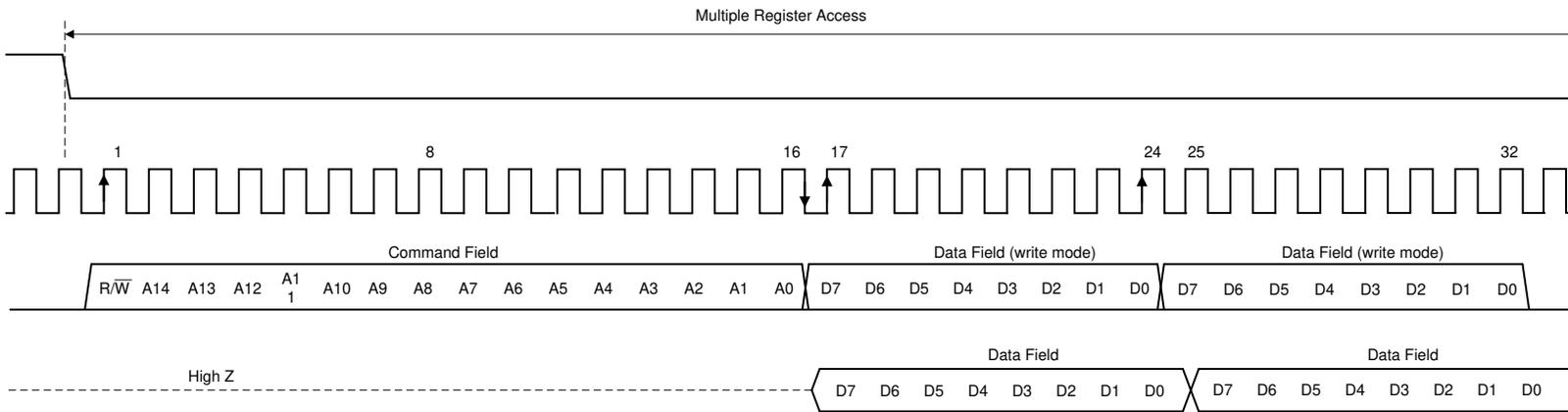
**Figure 6-6. Serial Interface Protocol: Streaming Read/Write Operation**
