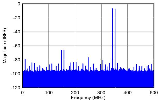
DES\_EN = 1,  $f_S = 1000\text{MHz}$ , FG calibration,  $f_1 = 342\text{MHz}$ ,  $f_2 = 352\text{MHz}$ ,  $A_{IN} = -7\text{dBFS}$  per tone, SFDR =  $-66\text{dBFS}$ , IMD3 =  $-85\text{dBFS}$ , IMD2 =  $-80\text{dBFS}$
