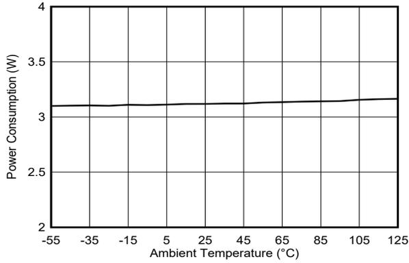
DES\_EN = 0,  $f_S = 2500\text{MHz}$ ,  $F_{IN} = 99\text{MHz}$ ,  $A_{IN} = -1\text{dBFS}$
