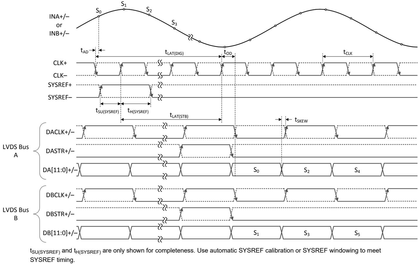
**Figure 5-5. Single-Channel, 2-Bus, Aligned-Mode Timing (LDEMUX = 0, DES\_EN = 1, LALIGNED = 1)**
