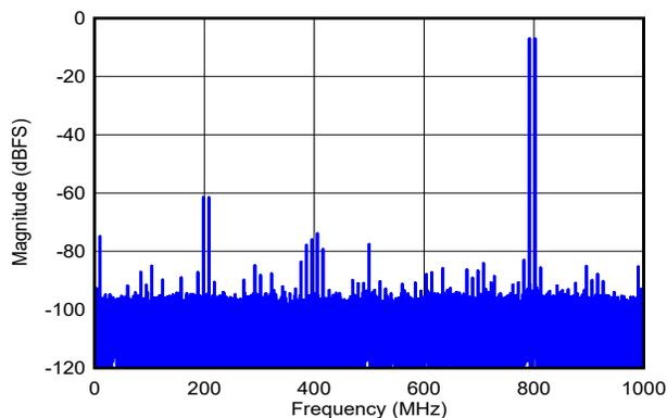
DES\_EN = 1,  $f_S = 2000\text{MHz}$ , FG calibration,  $f_1 = 792\text{MHz}$ ,  $f_2 = 802\text{MHz}$ ,  $A_{IN} = -7\text{dBFS}$  per tone, SFDR =  $-62\text{dBFS}$ , IMD3 =  $-84\text{dBFS}$ , IMD2 =  $-74\text{dBFS}$
