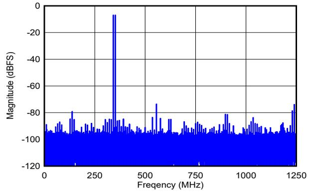
DES\_EN = 0,  $f_S = 2500\text{MHz}$ , FG calibration,  $f_1 = 342\text{MHz}$ ,  $f_2 = 352\text{MHz}$ ,  $A_{IN} = -7\text{dBFS}$  per tone, SFDR =  $-74\text{dBFS}$ , IMD3 =  $-86\text{dBFS}$ , IMD2 =  $-88\text{dBFS}$
