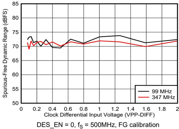
**Figure 5-36. SFDR vs Clock Amplitude**
