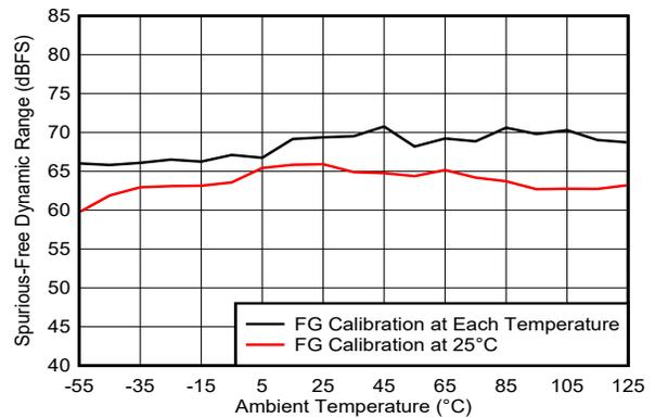
Figure 5-275. SFDR vs Temperature and Calibration Mode
