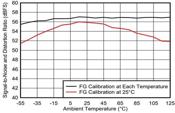
Figure 5-54. SINAD vs Temperature and Calibration Mode
