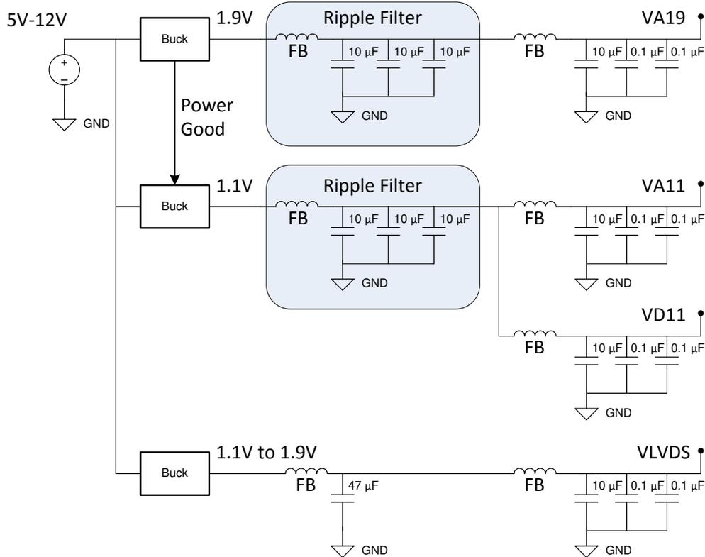
Ripple Filter Notch Frequency to Match  $f_s$  of Buck Converter
