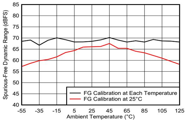
Figure 5-274. SFDR vs Temperature and Calibration Mode
