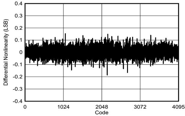
DES\_EN = 0,  $f_S = 1500\text{MHz}$ , FG calibration,  $F_{IN} = 99\text{MHz}$
