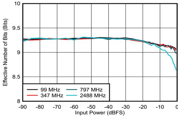
DES\_EN = 0,  $f_S = 2500\text{MHz}$ , FG calibration
