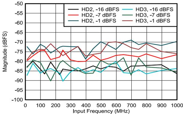
DES\_EN = 0,  $f_S = 1000\text{MHz}$ , FG calibration
