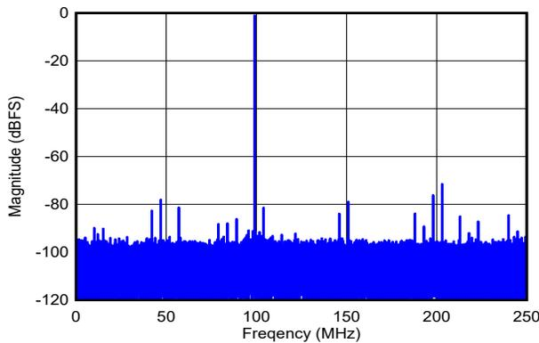
**Figure 5-38. Single-Tone FFT at  $f_{IN} = 99\text{MHz}$ ,  $A_{IN} = -1\text{dBFS}$**
