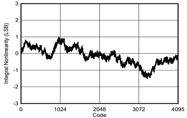
DES\_EN = 0,  $f_s = 2000\text{MHz}$ , FG calibration,  $F_{\text{IN}} = 99\text{MHz}$
