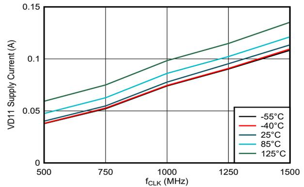
DES\_EN = 1,  $f_S = 3000\text{MHz}$ ,  $F_{IN} = 347\text{MHz}$ ,  $A_{IN} = -1\text{dBFS}$
