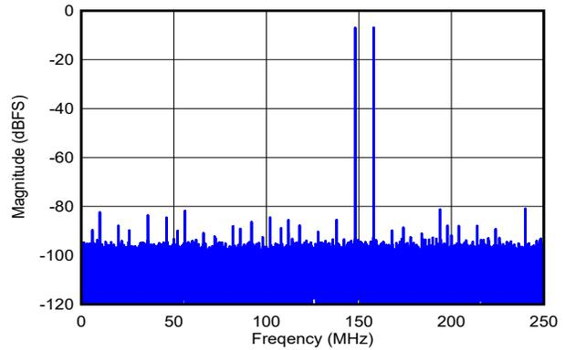
DES\_EN = 0,  $f_S = 500\text{MHz}$ , FG calibration,  $f_1 = 342\text{MHz}$ ,  $f_2 = 352\text{MHz}$ ,  $A_{IN} = -7\text{dBFS}$  per tone, SFDR =  $-81\text{dBFS}$ , IMD3 =  $-87\text{dBFS}$ , IMD2 =  $-82\text{dBFS}$
