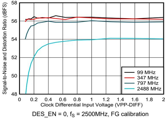
Figure 5-240. SINAD vs Clock Amplitude
