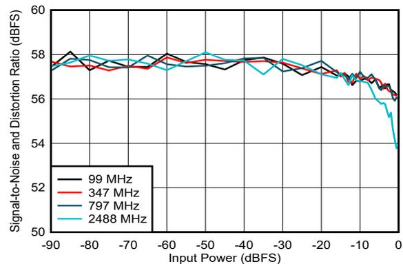
DES\_EN = 1,  $f_S = 3000\text{MHz}$ , FG calibration
