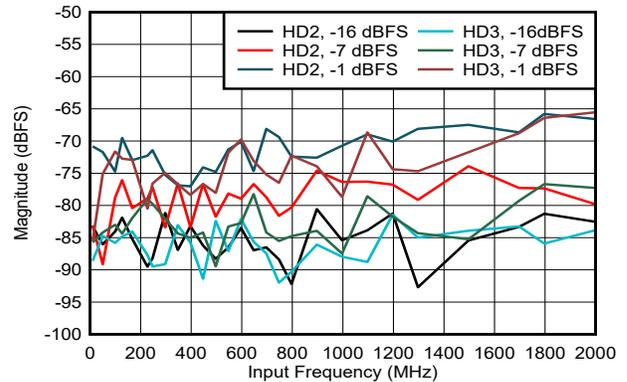
DES\_EN = 1,  $f_S = 2000\text{MHz}$ , FG calibration
