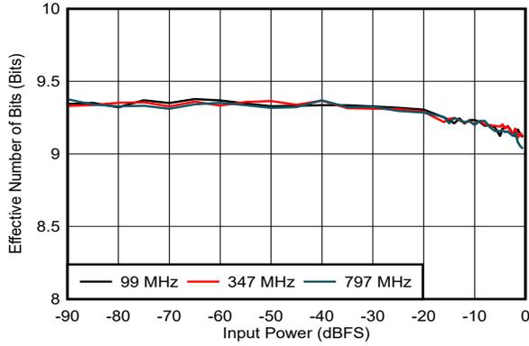
DES\_EN = 0,  $f_s = 1500\text{MHz}$ , FG calibration
