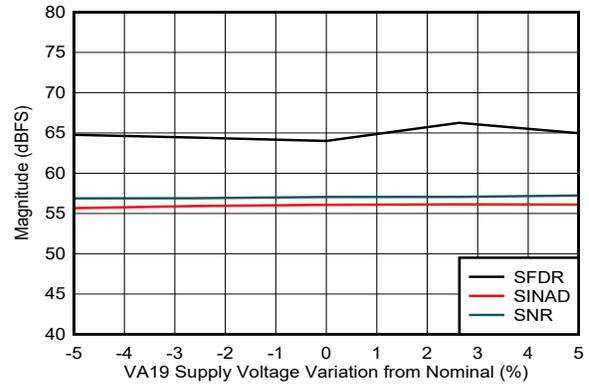
DES\_EN = 1,  $f_S = 1000\text{MHz}$ ,  $F_{IN} = 347\text{MHz}$ ,  $A_{IN} = -1\text{dBFS}$
