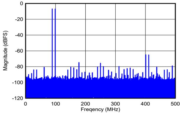
DES\_EN = 1,  $f_S = 1000\text{MHz}$ , FG calibration,  $f_1 = 89\text{MHz}$ ,  $f_2 = 99\text{MHz}$ ,  $A_{IN} = -7\text{dBFS}$  per tone, SFDR =  $-65\text{dBFS}$ , IMD3 =  $-95\text{dBFS}$ , IMD2 =  $-89\text{dBFS}$
