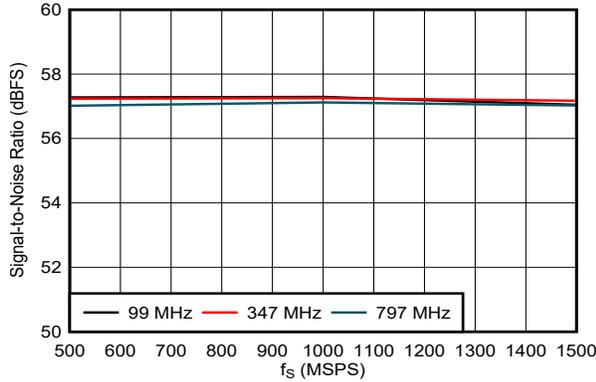
DES\_EN = 0,  $f_S = 1500\text{MHz}$ , FG calibration
