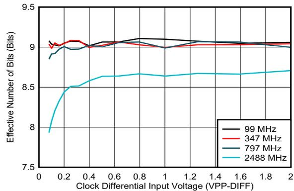
Figure 5-131. ENOB vs Clock Amplitude
