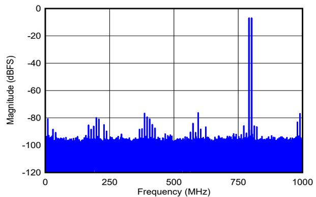
DES\_EN = 0,  $f_S = 2000\text{MHz}$ , FG calibration,  $f_1 = 792\text{MHz}$ ,  $f_2 = 802\text{MHz}$ ,  $A_{IN} = -7\text{dBFS}$  per tone, SFDR =  $-76\text{dBFS}$ , IMD3 =  $-88\text{dBFS}$ , IMD2 =  $-81\text{dBFS}$
