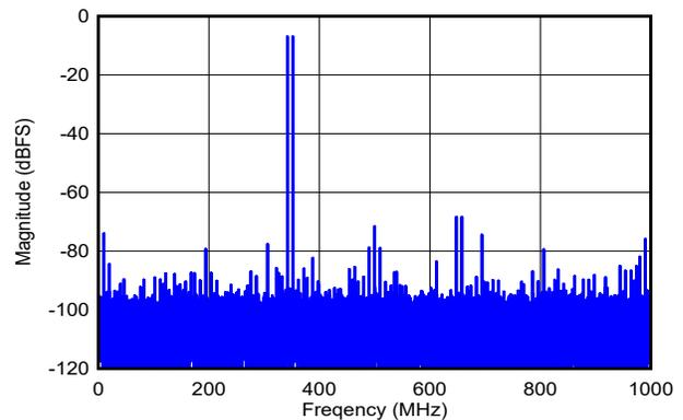
DES\_EN = 1,  $f_S = 2000\text{MHz}$ , FG calibration,  $f_1 = 342\text{MHz}$ ,  $f_2 = 352\text{MHz}$ ,  $A_{IN} = -7\text{dBFS}$  per tone, SFDR =  $-68\text{dBFS}$ , IMD3 =  $-89\text{dBFS}$ , IMD2 =  $-74\text{dBFS}$
