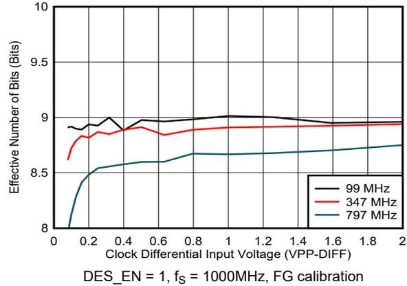
**Figure 5-35. ENOB vs Clock Amplitude**
