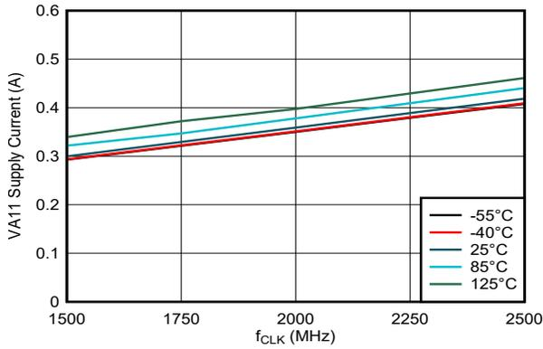
DES\_EN = 0,  $f_S = 2500\text{MHz}$ ,  $F_{IN} = 347\text{MHz}$ ,  $A_{IN} = -1\text{dBFS}$
