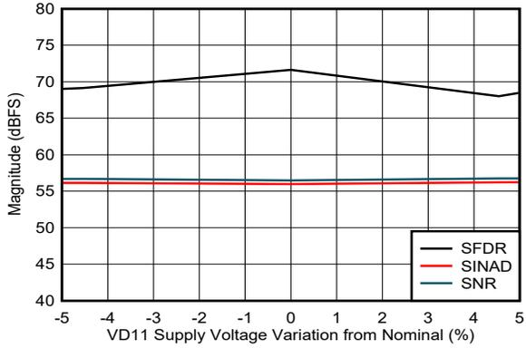
DES\_EN = 0,  $f_S = 2500\text{MHz}$ ,  $F_{IN} = 347\text{MHz}$ ,  $A_{IN} = -1\text{dBFS}$
