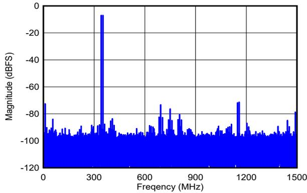
DES\_EN = 1,  $f_S = 3000\text{MHz}$ , FG calibration,  $f_1 = 342\text{MHz}$ ,  $f_2 = 352\text{MHz}$ ,  $A_{IN} = -7\text{dBFS}$  per tone, SFDR =  $-71\text{dBFS}$ , IMD3 =  $-88\text{dBFS}$ , IMD2 =  $-73\text{dBFS}$
