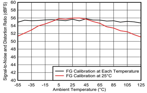
Figure 5-55. SINAD vs Temperature and Calibration Mode
