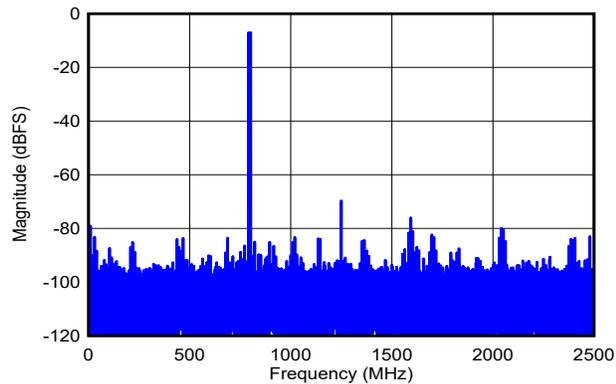
DES\_EN = 1,  $f_S = 5000\text{MHz}$ , FG calibration,  $f_1 = 792\text{MHz}$ ,  $f_2 = 802\text{MHz}$ ,  $A_{IN} = -7\text{dBFS}$  per tone, SFDR =  $-76\text{dBFS}$ , IMD3 =  $-93\text{dBFS}$ , IMD2 =  $-77\text{dBFS}$
