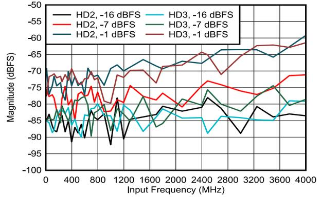
DES\_EN = 1,  $f_S = 4000\text{MHz}$ , FG calibration
