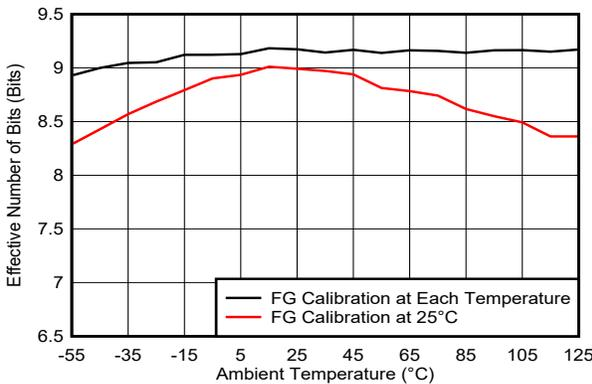
Figure 5-56. ENOB vs Temperature and Calibration Mode
