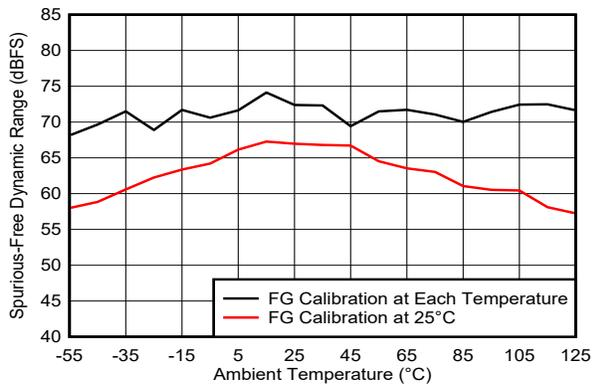
Figure 5-58. SFDR vs Temperature and Calibration Mode
