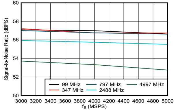
DES\_EN = 1,  $f_S = 5000\text{MHz}$ , FG calibration
