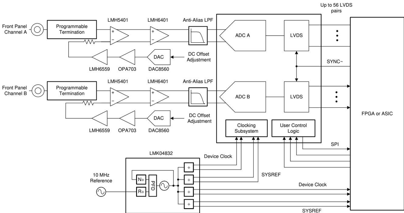
**Figure 7-1. Typical Configuration for a Reconfigurable Oscilloscope**
