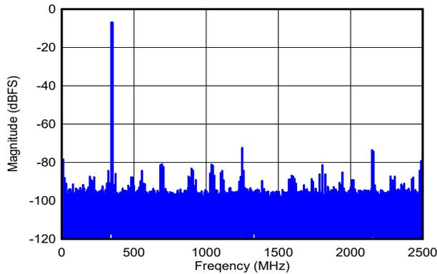
DES\_EN = 1,  $f_S = 5000\text{MHz}$ , FG calibration,  $f_1 = 342\text{MHz}$ ,  $f_2 = 352\text{MHz}$ ,  $A_{IN} = -7\text{dBFS}$  per tone, SFDR =  $-74\text{dBFS}$ , IMD3 =  $-91\text{dBFS}$ , IMD2 =  $-80\text{dBFS}$
