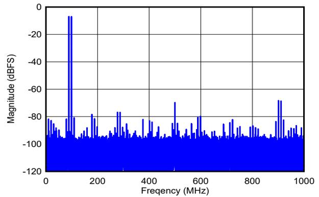
DES\_EN = 1,  $f_S = 2000\text{MHz}$ , FG calibration,  $f_1 = 89\text{MHz}$ ,  $f_2 = 99\text{MHz}$ ,  $A_{IN} = -7\text{dBFS}$  per tone, SFDR =  $-68\text{dBFS}$ , IMD3 =  $-81\text{dBFS}$ , IMD2 =  $-82\text{dBFS}$
