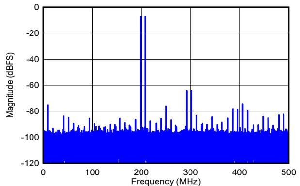
DES\_EN = 1,  $f_S = 1000\text{MHz}$ , FG calibration,  $f_1 = 792\text{MHz}$ ,  $f_2 = 802\text{MHz}$ ,  $A_{IN} = -7\text{dBFS}$  per tone, SFDR =  $-64\text{dBFS}$ , IMD3 =  $-87\text{dBFS}$ , IMD2 =  $-75\text{dBFS}$
