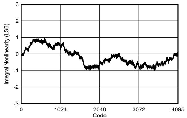
DES\_EN = 1,  $f_S = 3000\text{MHz}$ , FG calibration,  $F_{IN} = 99\text{MHz}$
