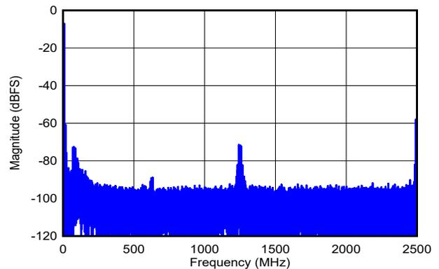
DES\_EN = 1,  $f_S = 5000\text{MHz}$ , FG calibration,  $f_1 = 4992\text{MHz}$ ,  $f_2 = 5002\text{MHz}$ ,  $A_{IN} = -7\text{dBFS}$  per tone, SFDR =  $-58\text{dBFS}$ , IMD3 =  $-61\text{dBFS}$ , IMD2 =  $-78\text{dBFS}$
