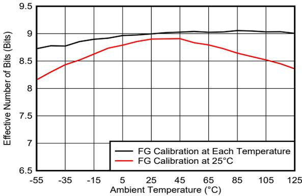
Figure 5-272. ENOB vs Temperature and Calibration Mode
