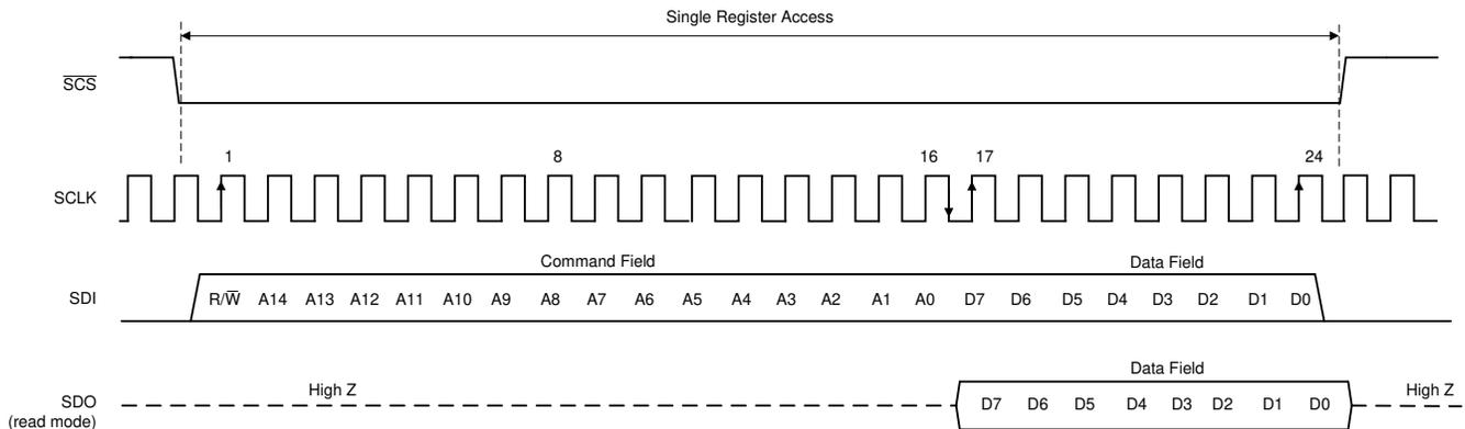
**Figure 6-5. Serial Interface Protocol: Single Read/Write Operation**
