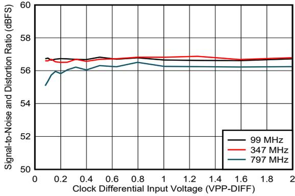
Figure 5-128. SINAD vs Clock Amplitude
