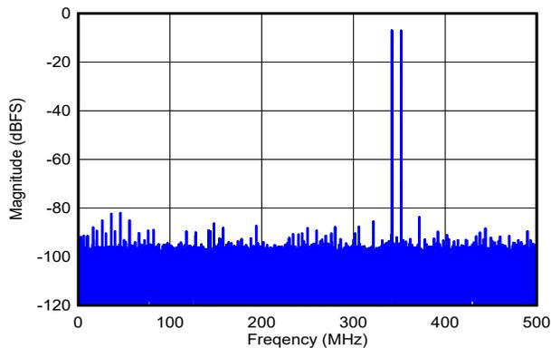
DES\_EN = 0,  $f_S = 1000\text{MHz}$ , FG calibration,  $f_1 = 342\text{MHz}$ ,  $f_2 = 352\text{MHz}$ ,  $A_{IN} = -7\text{dBFS}$  per tone, SFDR =  $-82\text{dBFS}$ , IMD3 =  $-96\text{dBFS}$ , IMD2 =  $-89\text{dBFS}$
