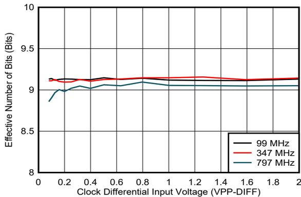
Figure 5-130. ENOB vs Clock Amplitude
