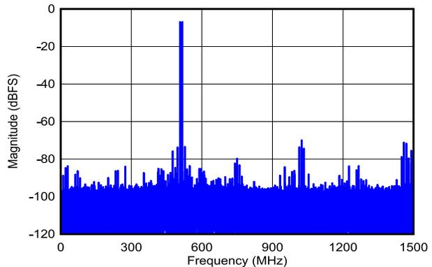
DES\_EN = 1,  $f_S = 3000\text{MHz}$ , FG calibration,  $f_1 = 2483\text{MHz}$ ,  $f_2 = 2493\text{MHz}$ ,  $A_{IN} = -7\text{dBFS}$  per tone, SFDR =  $-70\text{dBFS}$ , IMD3 =  $-74\text{dBFS}$ , IMD2 =  $-75\text{dBFS}$
