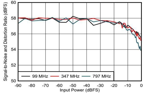
DES\_EN = 1,  $f_S = 1000\text{MHz}$ , FG calibration
