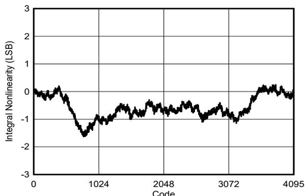
DES\_EN = 0,  $f_S = 1000\text{MHz}$ , FG calibration,  $F_{IN} = 99\text{MHz}$
