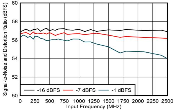
DES\_EN = 0,  $f_S = 2500\text{MHz}$ , FG calibration
