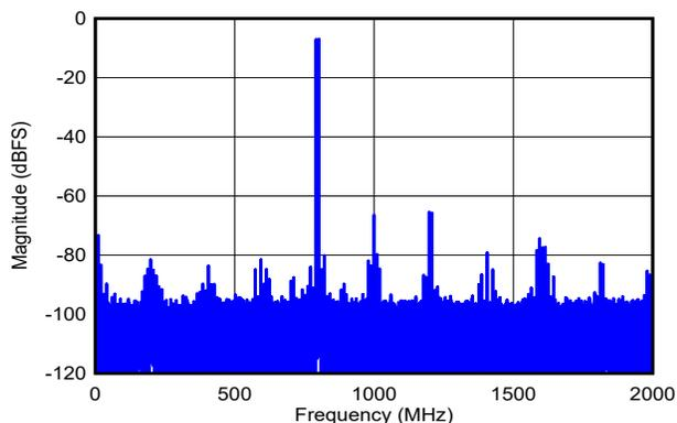
DES\_EN = 1,  $f_S = 4000\text{MHz}$ , FG calibration,  $f_1 = 792\text{MHz}$ ,  $f_2 = 802\text{MHz}$ ,  $A_{IN} = -7\text{dBFS}$  per tone, SFDR =  $-65\text{dBFS}$ , IMD3 =  $-87\text{dBFS}$ , IMD2 =  $-74\text{dBFS}$
