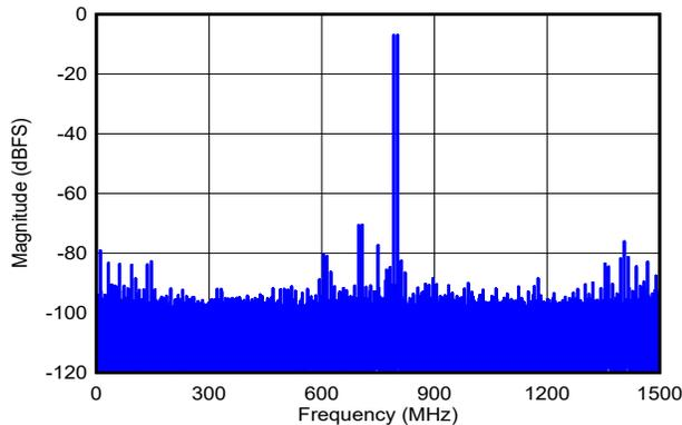
DES\_EN = 1,  $f_S = 3000\text{MHz}$ , FG calibration,  $f_1 = 792\text{MHz}$ ,  $f_2 = 802\text{MHz}$ ,  $A_{IN} = -7\text{dBFS}$  per tone, SFDR =  $-71\text{dBFS}$ , IMD3 =  $-84\text{dBFS}$ , IMD2 =  $-77\text{dBFS}$
