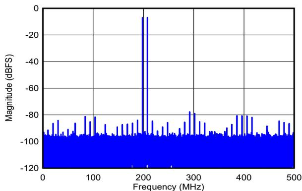
DES\_EN = 0,  $f_S = 1000\text{MHz}$ , FG calibration,  $f_1 = 792\text{MHz}$ ,  $f_2 = 802\text{MHz}$ ,  $A_{IN} = -7\text{dBFS}$  per tone, SFDR =  $-78\text{dBFS}$ , IMD3 =  $-84\text{dBFS}$ , IMD2 =  $-85\text{dBFS}$
