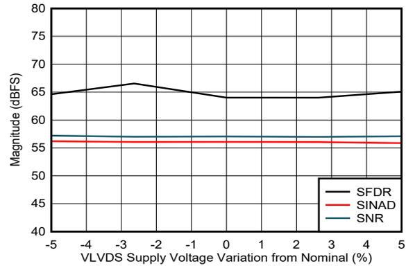
DES\_EN = 1,  $f_S = 1000\text{MHz}$ ,  $F_{IN} = 347\text{MHz}$ ,  $A_{IN} = -1\text{dBFS}$
