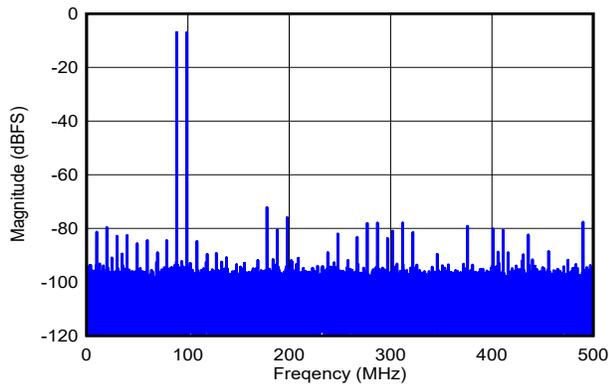
DES\_EN = 0,  $f_S = 1000\text{MHz}$ , FG calibration,  $f_1 = 89\text{MHz}$ ,  $f_2 = 99\text{MHz}$ ,  $A_{IN} = -7\text{dBFS}$  per tone, SFDR =  $-72\text{dBFS}$ , IMD3 =  $-85\text{dBFS}$ , IMD2 =  $-81\text{dBFS}$
