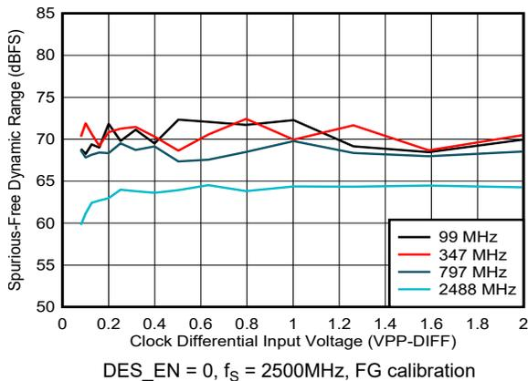
Figure 5-244. SFDR vs Clock Amplitude
