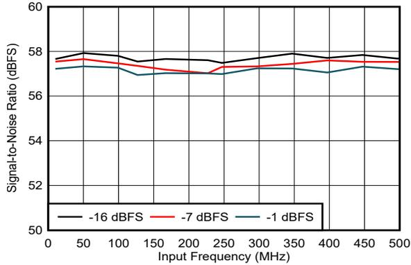
DES\_EN = 0,  $f_S = 500\text{MHz}$ , FG calibration
