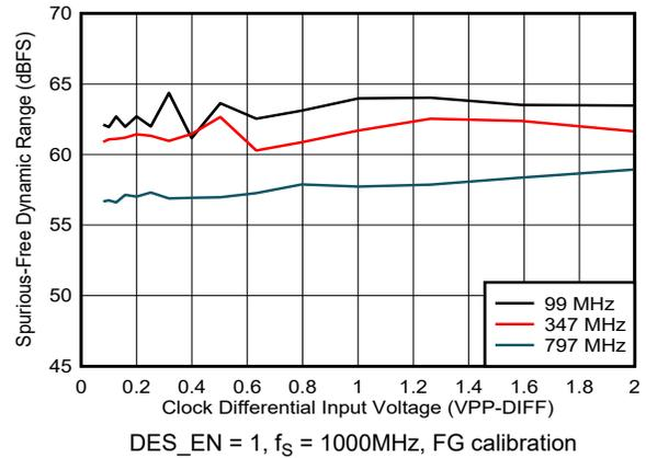
**Figure 5-37. SFDR vs Clock Amplitude**
