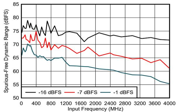
DES\_EN = 1,  $f_S = 4000\text{MHz}$ , FG calibration
