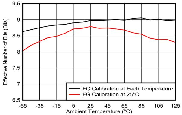
Figure 5-273. ENOB vs Temperature and Calibration Mode
