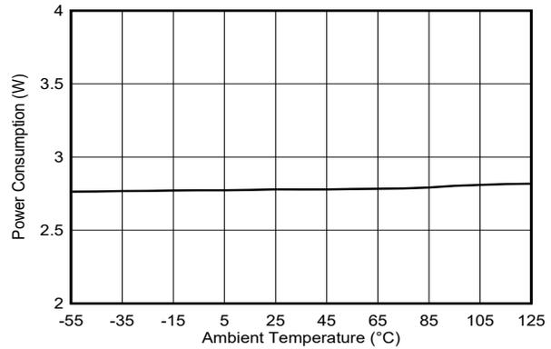
DES\_EN = 1,  $f_S = 3000\text{MHz}$ ,  $F_{IN} = 99\text{MHz}$ ,  $A_{IN} = -1\text{dBFS}$
