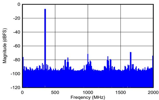
DES\_EN = 1,  $f_S = 4000\text{MHz}$ , FG calibration,  $f_1 = 342\text{MHz}$ ,  $f_2 = 352\text{MHz}$ ,  $A_{IN} = -7\text{dBFS}$  per tone, SFDR =  $-69\text{dBFS}$ , IMD3 =  $-95\text{dBFS}$ , IMD2 =  $-77\text{dBFS}$
