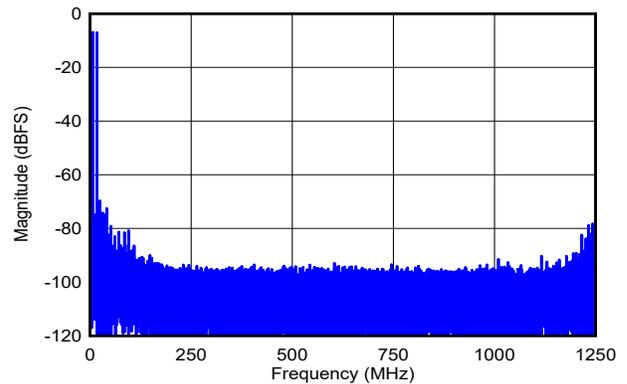
DES\_EN = 0,  $f_S = 2500\text{MHz}$ , FG calibration,  $f_1 = 2483\text{MHz}$ ,  $f_2 = 2493\text{MHz}$ ,  $A_{IN} = -7\text{dBFS}$  per tone, SFDR =  $-70\text{dBFS}$ , IMD3 =  $-76\text{dBFS}$ , IMD2 =  $-74\text{dBFS}$
