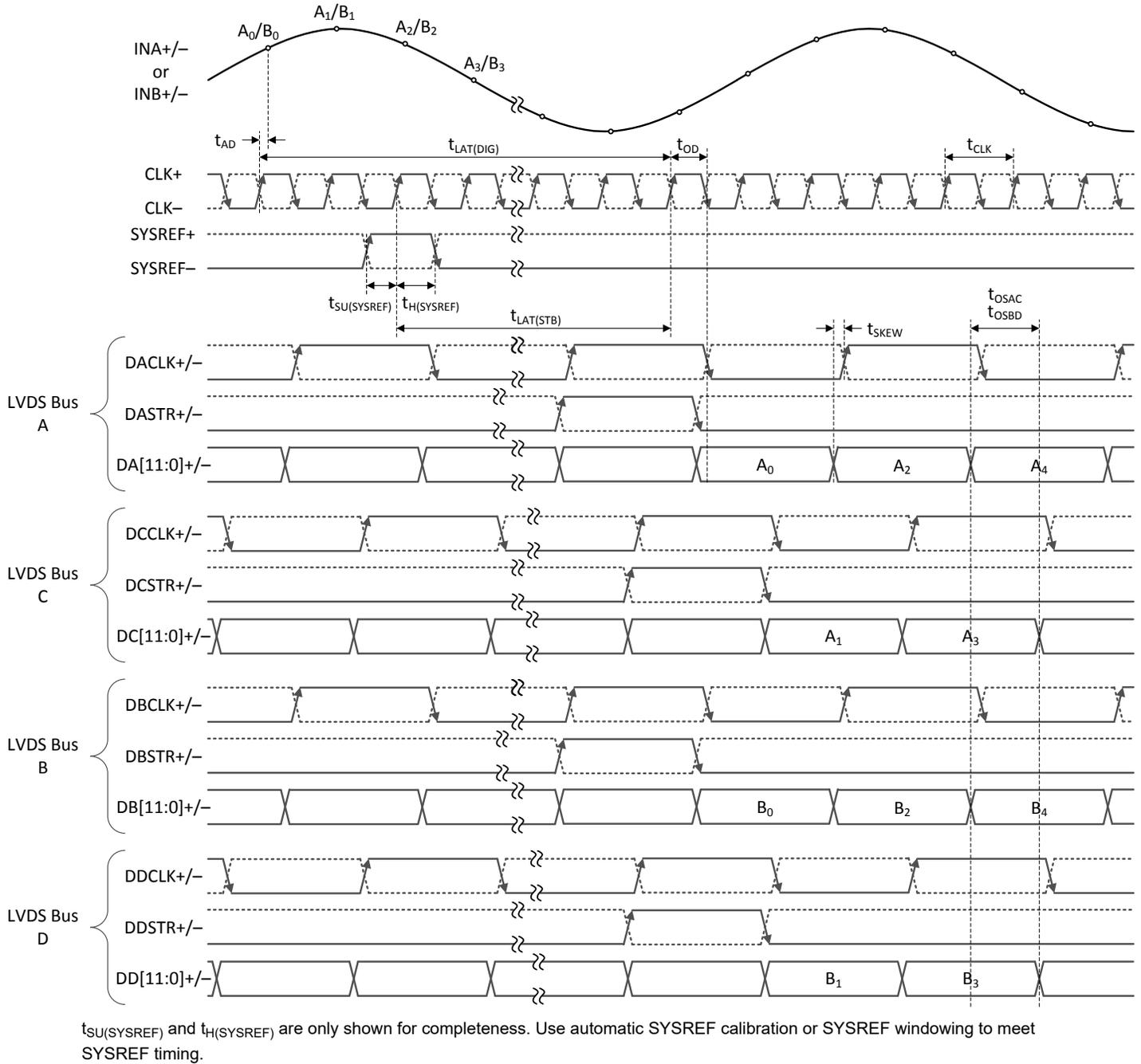
**Figure 5-2. Dual-Channel, 4-Bus, Staggered-Mode Timing (LDEMUX = 1, DES\_EN = 0, LALIGNED = 0)**
