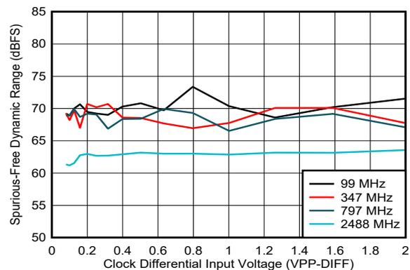
Figure 5-133. SFDR vs Clock Amplitude
