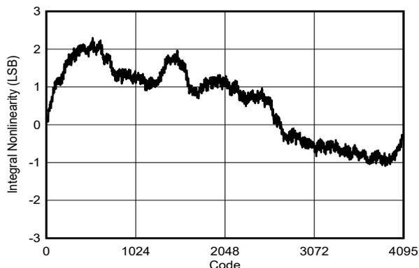
DES\_EN = 1,  $f_S = 5000\text{MHz}$ , FG calibration,  $F_{IN} = 99\text{MHz}$
