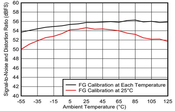
Figure 5-271. SINAD vs Temperature and Calibration Mode
