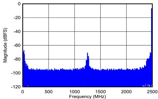
DES\_EN = 1,  $f_S = 5000\text{MHz}$ , FG calibration,  $f_1 = 2483\text{MHz}$ ,  $f_2 = 2493\text{MHz}$ ,  $A_{IN} = -7\text{dBFS}$  per tone, SFDR =  $-67\text{dBFS}$ , IMD3 =  $-74\text{dBFS}$ , IMD2 =  $-73\text{dBFS}$
