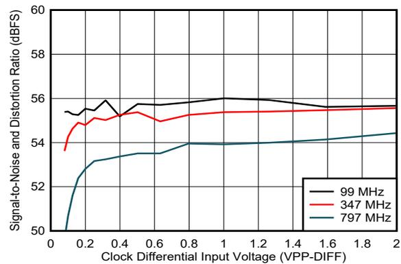
DES\_EN = 1,  $f_S = 1000\text{MHz}$ , FG calibration
