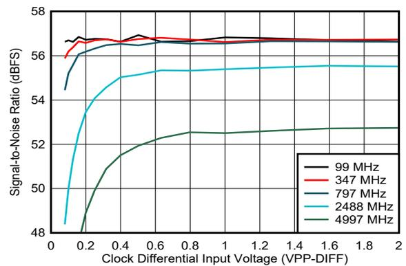
DES\_EN = 1,  $f_S = 5000\text{MHz}$ , FG calibration
