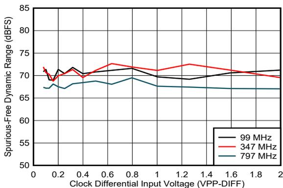
Figure 5-132. SFDR vs Clock Amplitude
