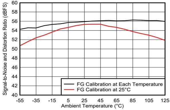
Figure 5-270. SINAD vs Temperature and Calibration Mode
