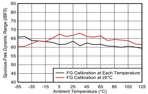
Figure 5-59. SFDR vs Temperature and Calibration Mode
