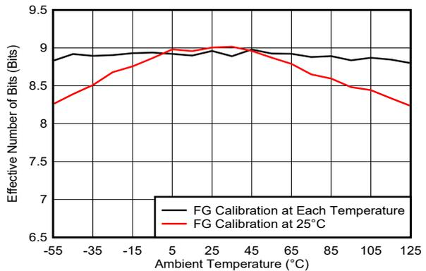
Figure 5-57. ENOB vs Temperature and Calibration Mode
