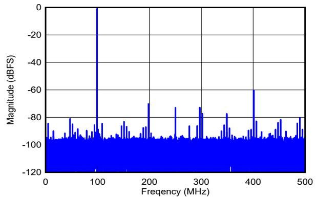
**Figure 5-39. Single-Tone FFT at  $f_{IN} = 99\text{MHz}$ ,  $A_{IN} = -1\text{dBFS}$**
