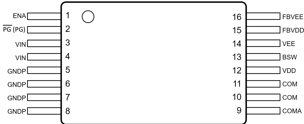
Figure 5-1. DHA Package, 16-Pin SSOP (Top View)
