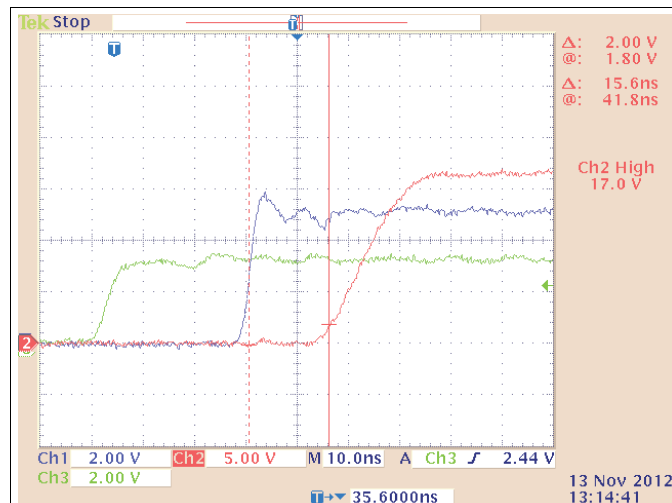
Figure 42. UCC27531DBV Input vs. Output PWM Propagation Delay (High)
