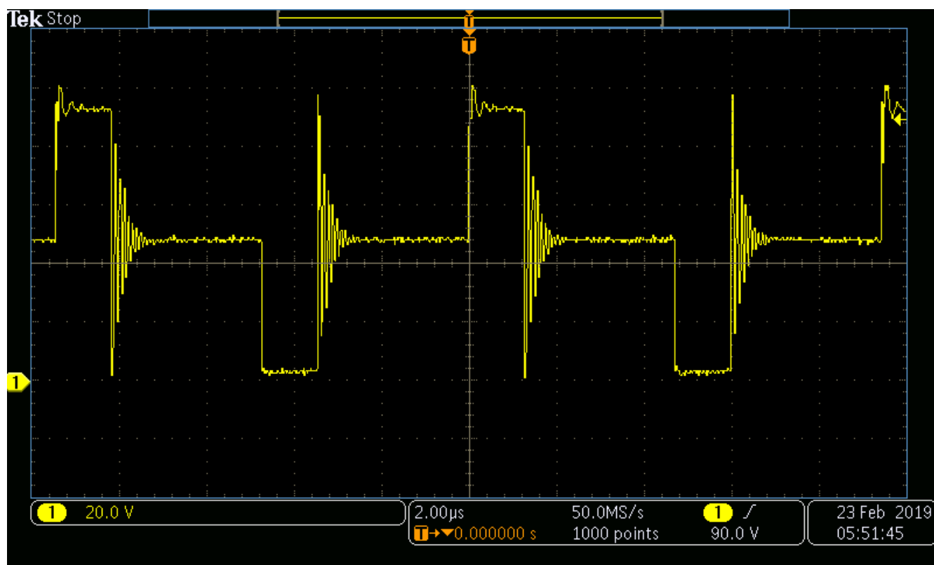
Figure 8-6. Voltage Stress Across Main Switching MOSFETS Q1 and Q2
