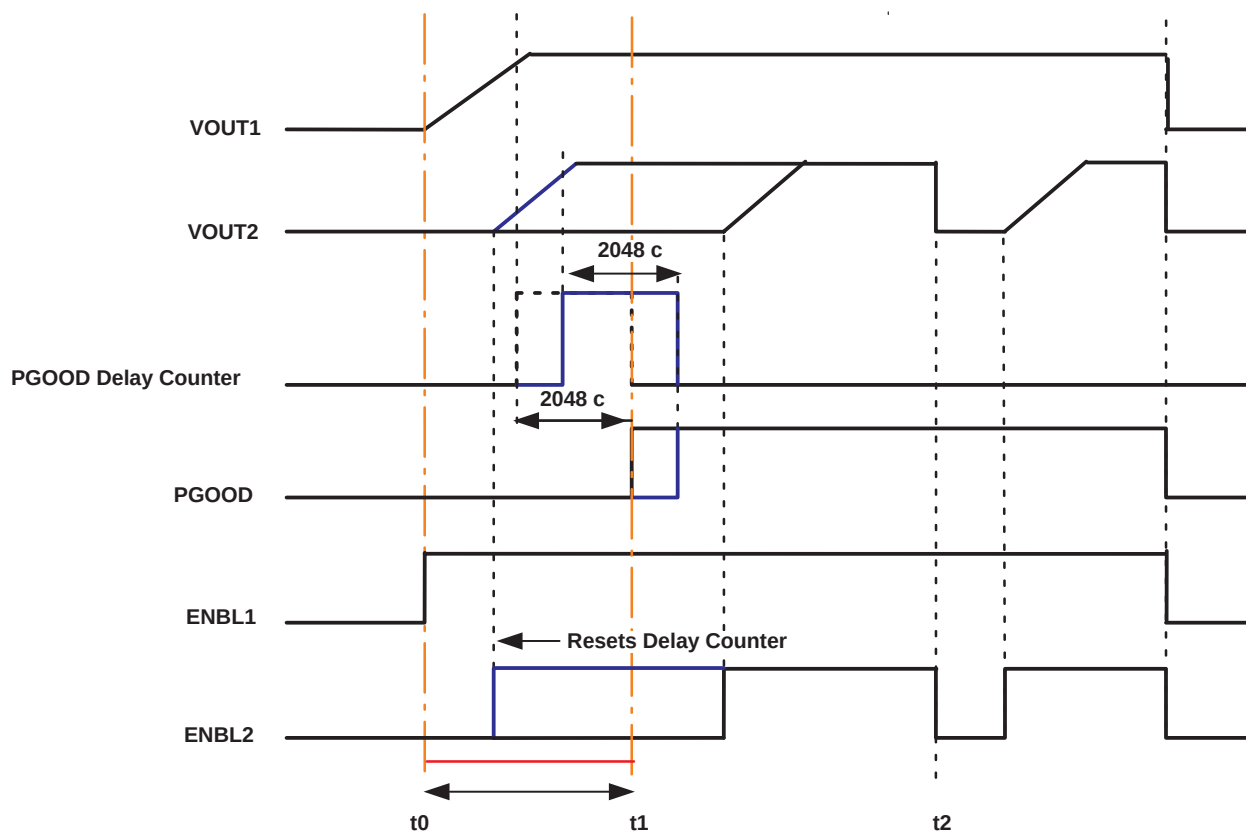
Figure 3. PowerGood Timing Diagram
