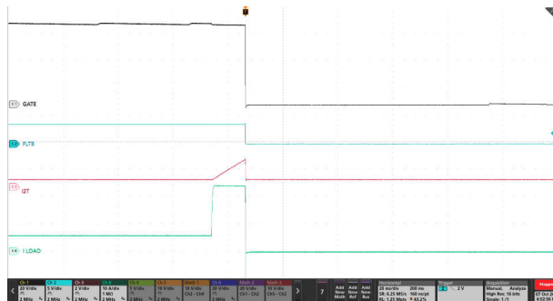
Figure 9-4. I^2T based Overcurrent Response of TPS4816-Q1 EVM for 6A to 23A Load Step
