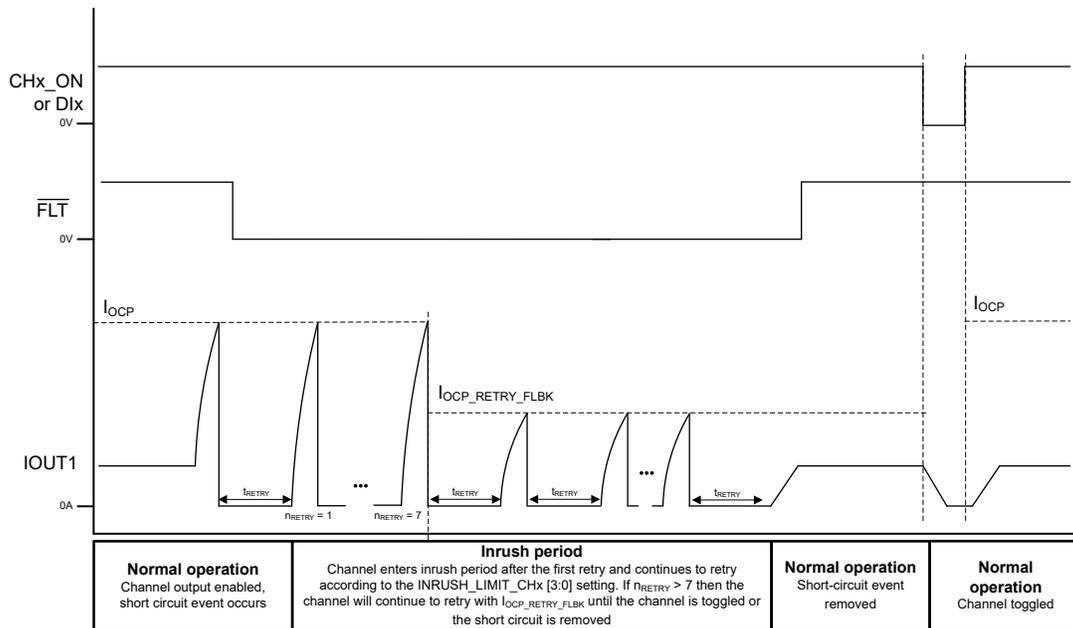
**Figure 8-25. Hot Short during Steady State Operation with CAP\_CHRG\_CHx = 00, Auto-retry (LATCH\_CHx = 0), and I<sub>OCP</sub> > I<sub>OCP\_RETRY\_FLBK</sub>**
