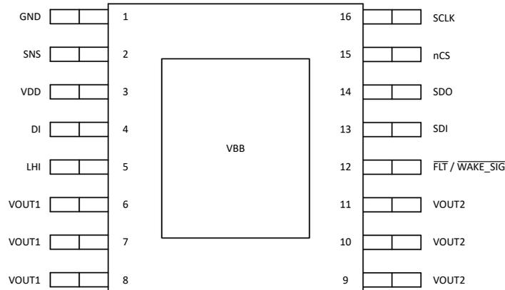
Figure 5-1. TPS2HCS08A-Q1 PWP Package,16-Pin HTSSOP (Top View)
