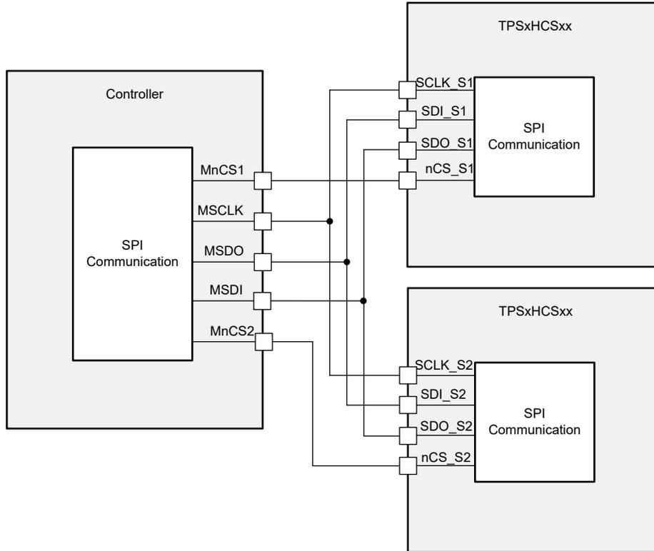
**Figure 8-6. Independent Secondary Configuration (Separate nCS Signal)**
