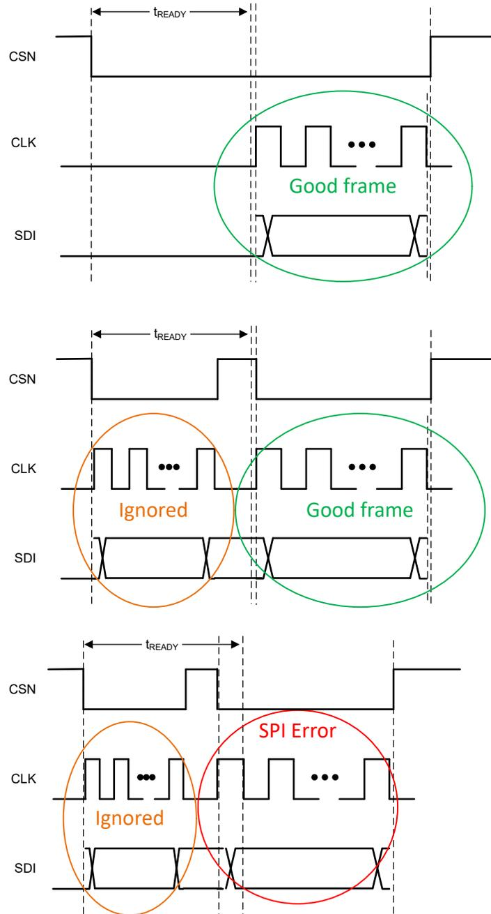
**Figure 8-13. Startup Communication Timing**
