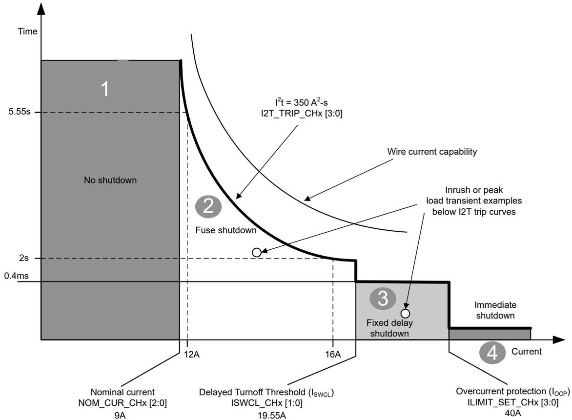
**Figure 8-23. Operational Region of Fuse Based Shutdown**
