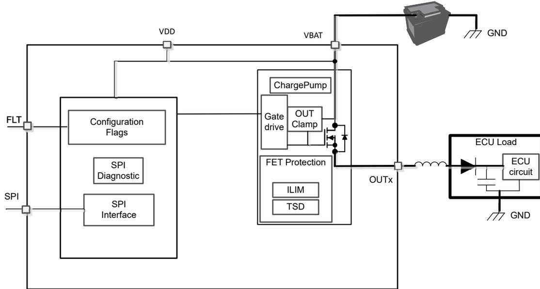
Figure 9-3. Block Diagram for Powering an ECU load with Input Capacitance
