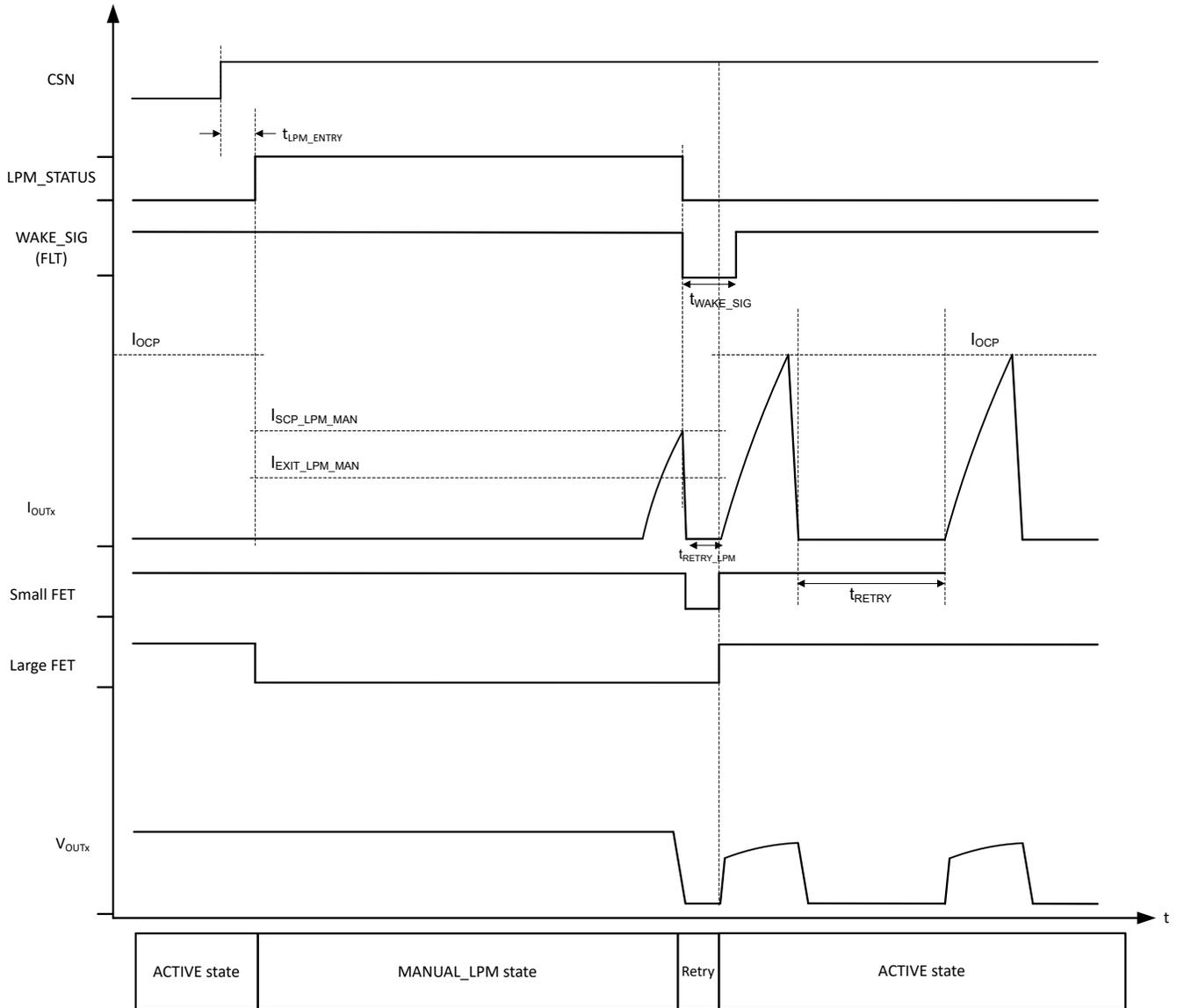
**Figure 8-16. Load Increase Above  $I_{OCP}$  in MANUAL\_LPM State**
