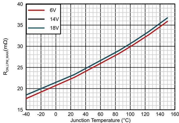
**Figure 6-5. On resistance in MANUAL\_LPM ( $R_{ON\_LPM\_MAN}$ ) vs Temperature**
