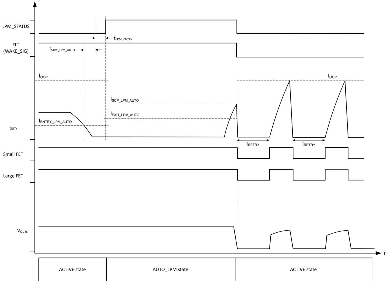
**Figure 8-19. Load Increase Above  $I_{OCP}$  in AUTO\_LPM State**
