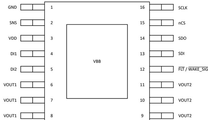
**Figure 5-2. PWP Package, 16-Pin HTSSOP (Top View) - TPS2HCS08B-Q1**
