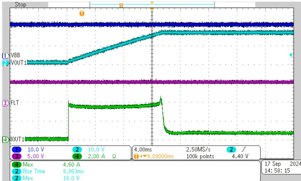
**Figure 9-4. I<sub>CL\_REG</sub> - Current Limit Regulation, V<sub>BB</sub> = 16V, T<sub>AMB</sub> = 105C, INRUSH\_DURATION = 0x7 (100ms), INRUSH\_LIMIT\_CHx = 0x6 (4.2A)**
