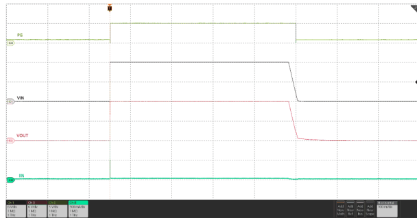
V_{EN/UVLO} = 2\text{ V} , C_{OUT} = 22\text{ }\mu\text{F} , C_{dVdt} = \text{Open} , V_{IN} ramped from 0\text{ V} \rightarrow 12\text{ V} \rightarrow 0\text{ V}
