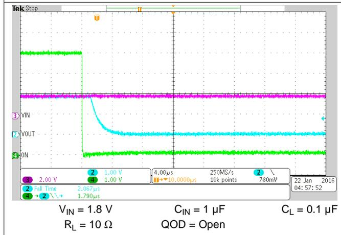
Figure 18. Fall Time ( $t_F$ ) at  $V_{IN} = 1.8\text{ V}$
