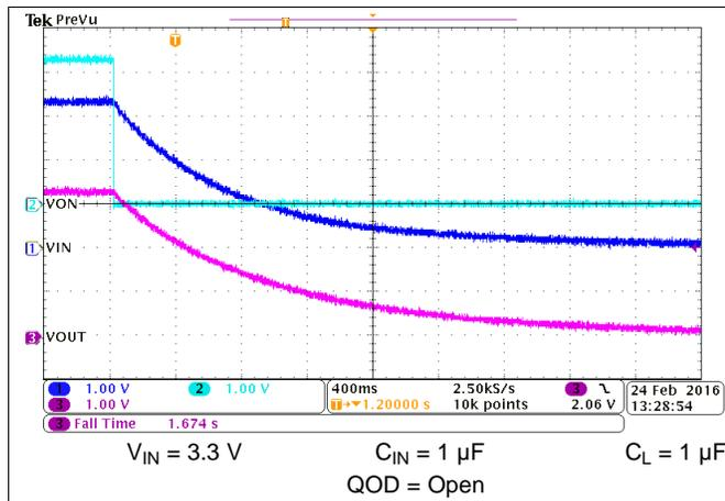
Figure 24. Fall Time ( $t_F$ ) at  $V_{IN} = 3.3 V$
