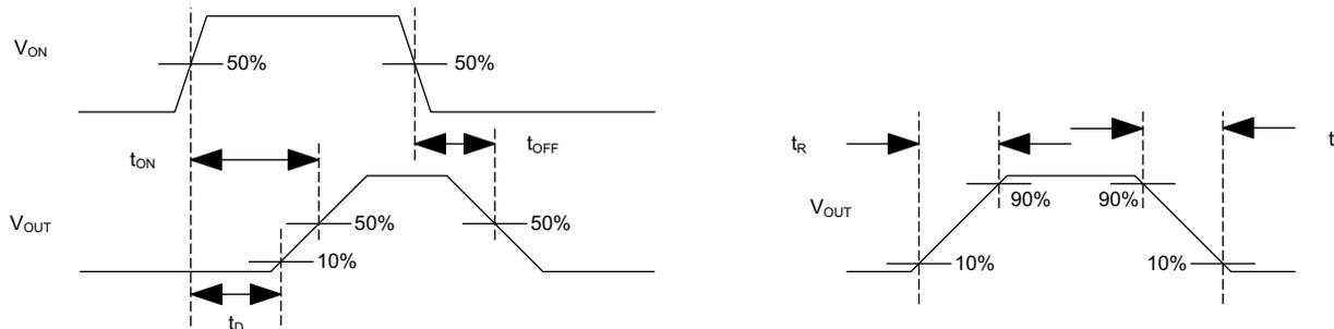
Figure 22. Timing Waveforms
