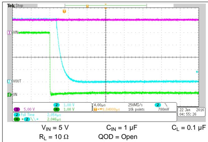
Figure 14. Fall Time ( $t_F$ ) at  $V_{IN} = 5\text{ V}$
