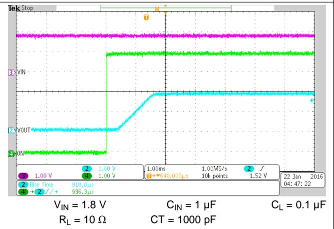
Figure 17. Rise Time ( $t_R$ ) at  $V_{IN} = 1.8\text{ V}$
