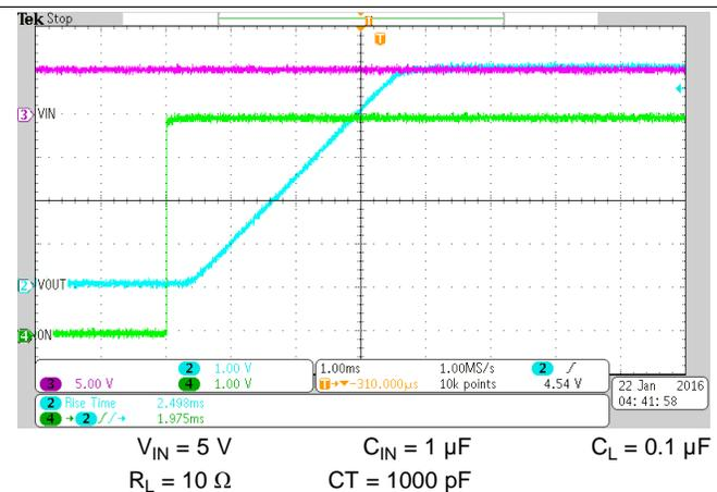
Figure 13. Rise Time ( $t_R$ ) at  $V_{IN} = 5 V$
