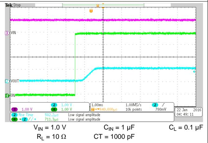
Figure 19. Rise Time ( $t_R$ ) at  $V_{IN} = 1\text{ V}$
