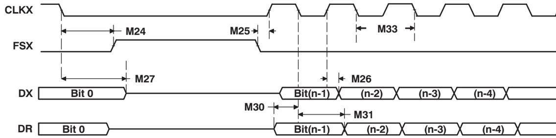
Figure 5-42. ASP as SPI: CLKSTP = 10b, CLKXP = 0
