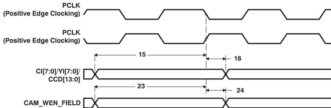
Figure 5-25. VPFE (CCD) Master Mode Input Data Timing
