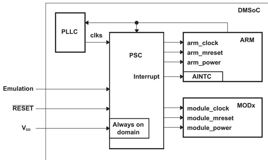
Figure 3-5. DM355 Power and Sleep Controller (PSC)
