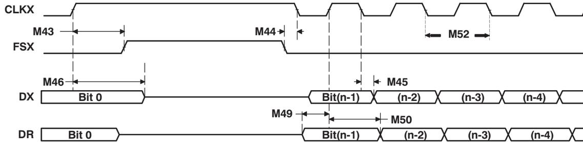
**Figure 5-44. ASP as SPI: CLKSTP = 10b, CLKXP = 1**
