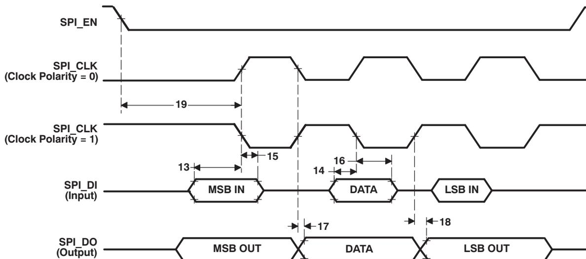
**Figure 5-38. SPI Master Mode External Timing (Clock Phase = 1)**
