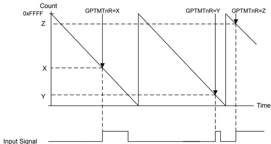
**Note:** When operating in Edge-time mode, the counter uses a modulo  $2^{24}$  count if prescaler is enabled or  $2^{16}$ , if not. If there is a possibility the edge could take longer than the count, then another timer configured in periodic-timer mode can be implemented to ensure detection of the missed edge. The periodic timer should be configured in such a way that:
