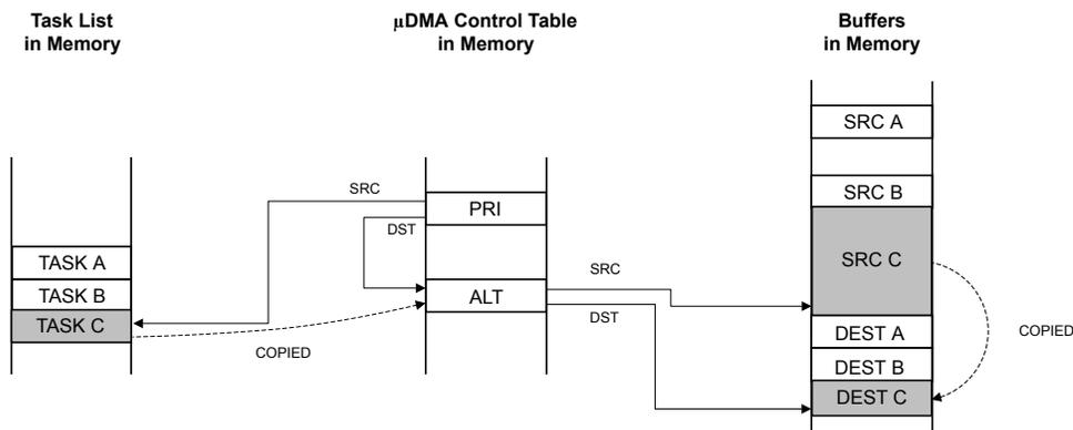
Using the channel's primary control structure, the  $\mu$ DMA controller copies task C configuration to the channel's alternate control structure.
