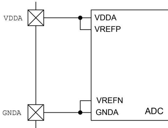
The range of this conversion value is from 0x000 to 0xFFF. In single-ended-input mode, the 0x000 value corresponds to the voltage level on VREFN; the 0xFFF value corresponds to the voltage level on VREFP. This configuration results in a resolution that can be calculated using the following equation:
