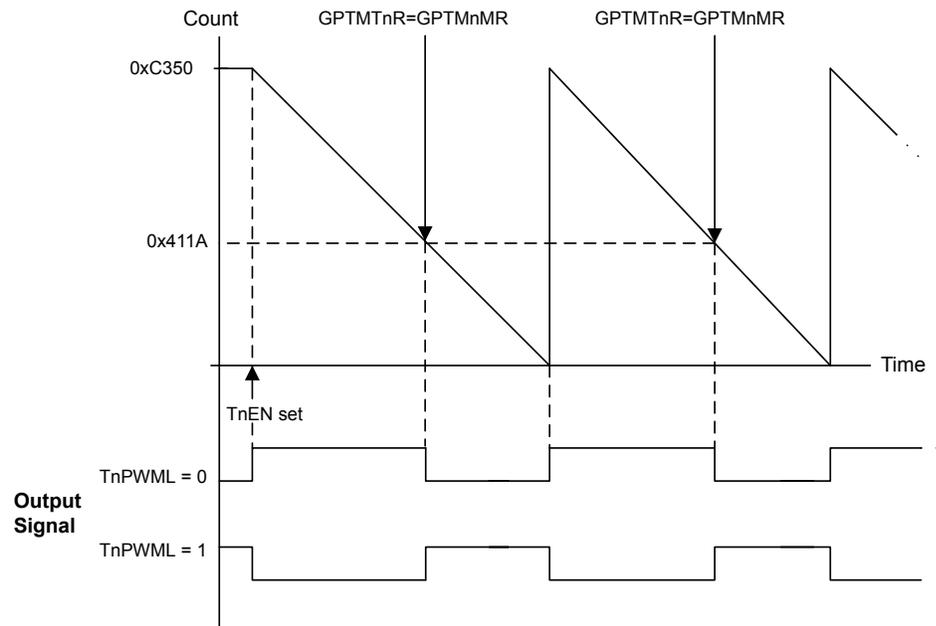
When synchronizing the timers using the **GPTMSYNC** register, the timer must be properly configured to avoid glitches on the CCP outputs. Both the  $TnPLO$  and the  $TnMRSU$  bits must be set in the **GPTMTnMR** register. Figure 10-6 on page 677 shows how the CCP output operates when the  $TnPLO$  and  $TnMRSU$  bits are set and the **GPTMTnMATCHHR** value is greater than the **GPTMTnILR** value.
