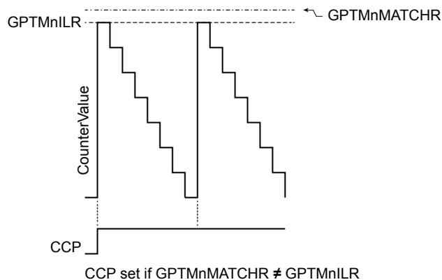
Figure 10-7 on page 678 shows how the CCP output operates when the  $PLO$  and  $MRSU$  bits are set and the **GPTMTnMATCHHR** value is the same as the **GPTMTnILR** value. In this situation, if the  $PLO$  bit is 0, the CCP signal goes high when the **GPTMTnILR** value is loaded and the match would be essentially ignored.
