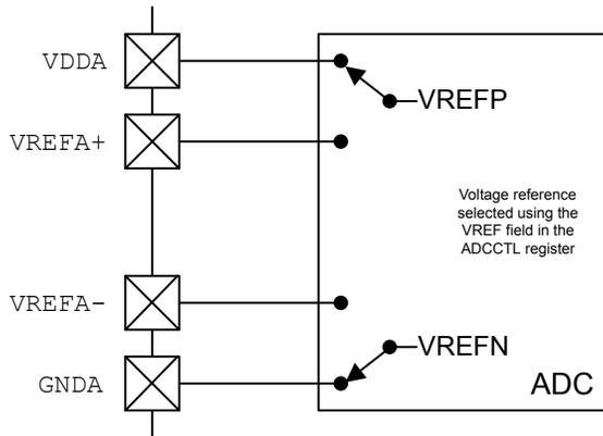
The range of this conversion value is from 0x000 to 0xFFFF. In single-ended-input mode, the 0x000 value corresponds to the voltage level on VREFN; the 0xFFFF value corresponds to the voltage level on VREFP. This configuration results in a resolution that can be calculated using the following equation:
