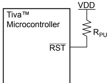
$R_{\text{PU}} = 0$  to 100 k $\Omega$
