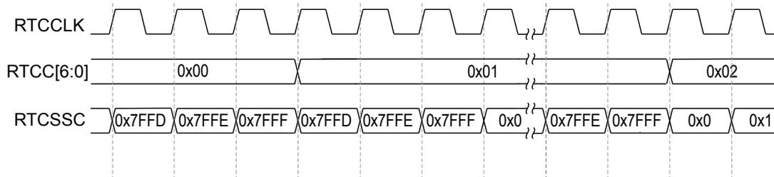
In the case of a trim value below `0x7FFF`, the `RTCSSC` value is advanced from `0x7FFF` to the trim value while the `RTCC` value is incremented from `0x0` to `0x1`. If the match value is within that range, the match interrupt is not triggered. For example, as shown in Figure 7-6 on page 483, if the match interrupt was configured with `RTCM0=0x1` and `RTCSSM=0x2`, an interrupt would never be triggered.
