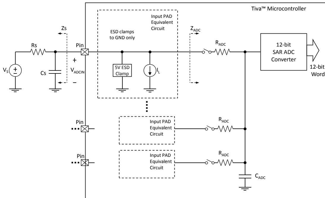
The ADC operates from both the 3.3-V analog and 1.2-V digital power supplies. The ADC clock can be configured to reduce power consumption when ADC conversions are not required (see “System Control” on page 219). The analog inputs are connected to the ADC through specially balanced input paths to minimize the distortion and cross-talk on the inputs. Detailed information on the ADC power supplies and analog inputs can be found in “Analog-to-Digital Converter (ADC)” on page 1223.
