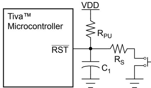
Typical  $R_{PU} = 10 \text{ k}\Omega$
