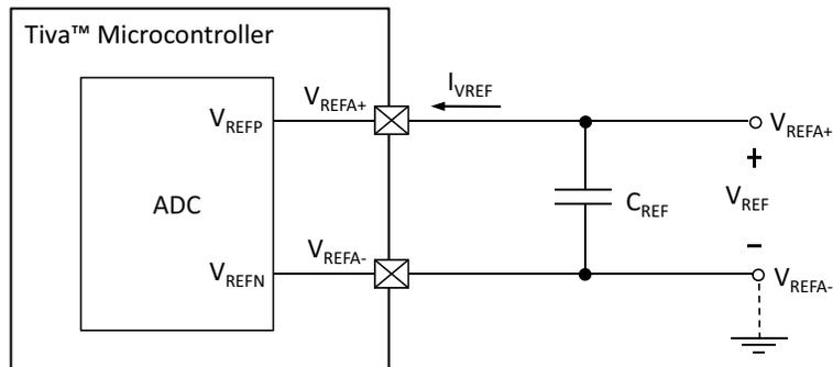
Figure 22-19. ADC Input Equivalency Diagram
