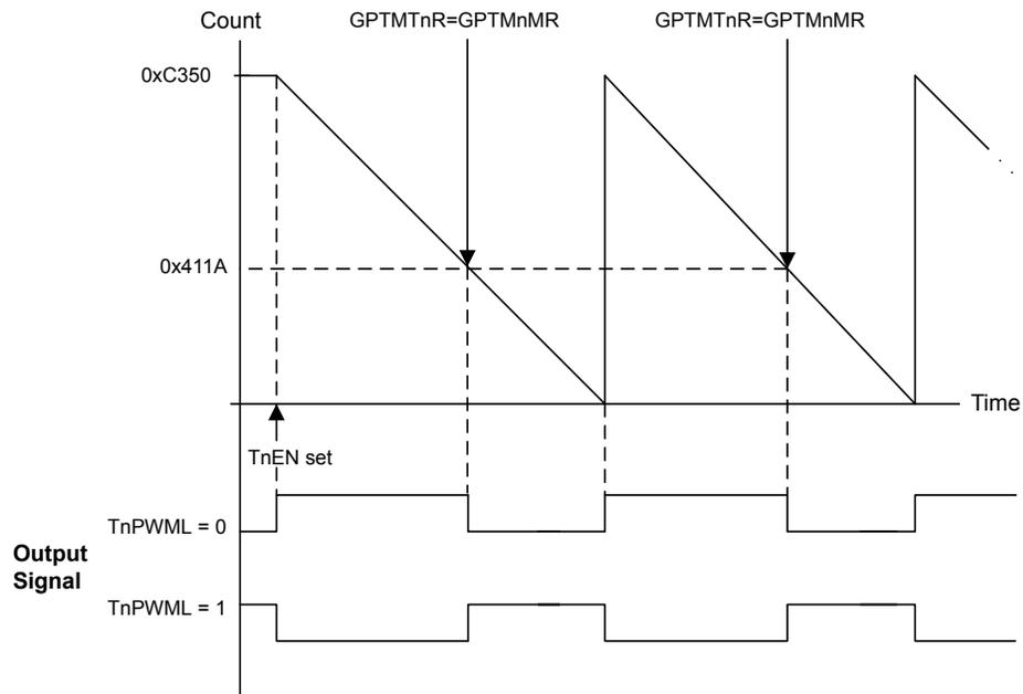
When synchronizing the timers using the **GPTMSYNC** register, the timer must be properly configured to avoid glitches on the CCP outputs. Both the  $TnPLO$  and the  $TnMRSU$  bits must be set in the **GPTMTnMR** register. Figure 11-6 on page 704 shows how the CCP output operates when the  $TnPLO$  and  $TnMRSU$  bits are set and the **GPTMTnMATCHR** value is greater than the **GPTMTnILR** value.
