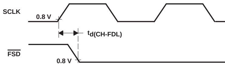
Figure 5-3. Master/Slave SCLK to \overline{FSD} Timing
