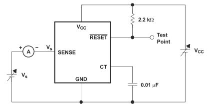
Figure 7-4.  $V_{s}$  and  $I_{s}$  Characteristics Measurement Circuit
