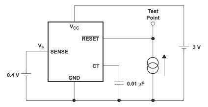
Figure 7-3.  $I_{OL}$  vs  $V_{OL}$  Measurement Circuit
