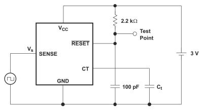
Figure 7-5. Switching Characteristics Measurement Circuit
