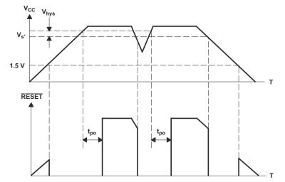
The desired sense voltage ( $V_{s'}$ ) is different from the SENSE input voltage ( $V_s$ ).  $V_s$  is typically 500 mV for triggering.
