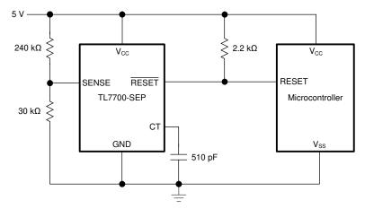
Figure 9-1. 5-V Supply Voltage Supervision
