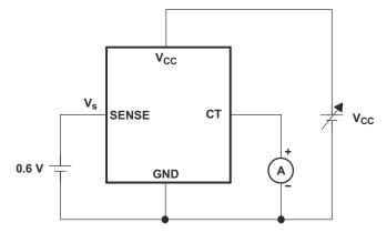
Figure 7-2. V<sub>CC</sub> vs I<sub>CT</sub> Measurement Circuit
