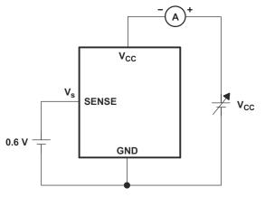
Figure 7-1.  $V_{CC} \mbox{ vs } I_{CC}$  Measurement Circuit
