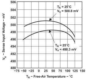
Figure 9-2. SENSE Input Voltage vs Temperature
