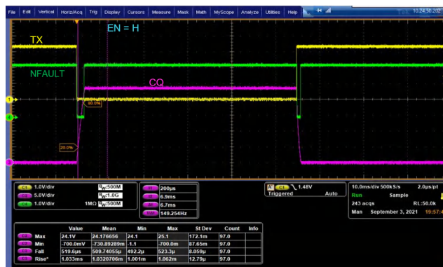
Figure 9-6. CQ Driving Inductive Load, Low Side Mode (NPN mode)
