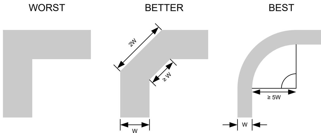
**Figure 8-2. Example Trace Corners for Improved Signal Integrity**
