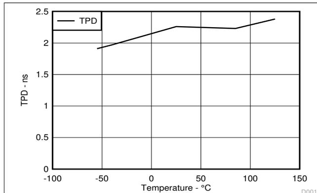
Figure 5-1. TPD Across Temperature at 3.3V Vcc
