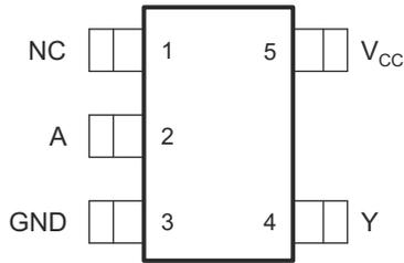
Figure 4-1. DBV Package 5-Pin SOT-23 Top View
