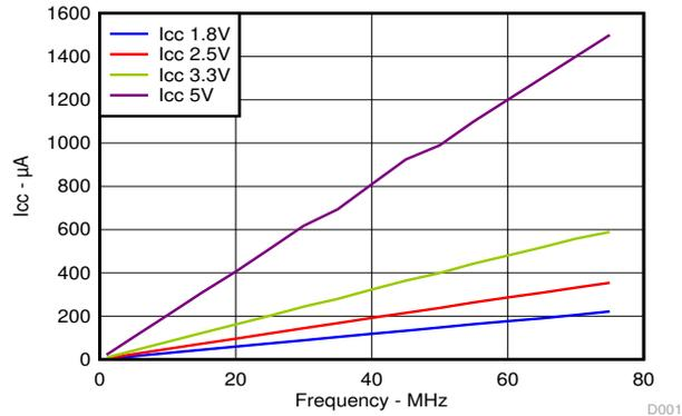
Figure 7-2. I<sub>CC</sub> vs Frequency
