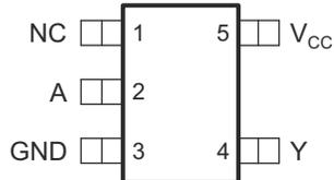
Figure 4-3. DCK Package 5-Pin SC70 Top View
