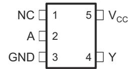
Figure 4-2. DRL Package 5-Pin SOT-5X3 Top View
