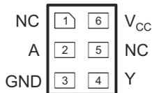
Figure 4-5. DRY Package 6-Pin SON Top View
