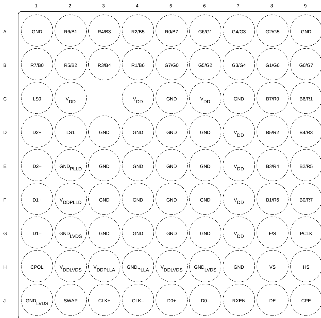
Figure 5-1. ZXH Package 80-Pin nFBGA Top View
