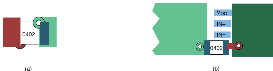
Figure 22. Typical Decoupling Capacitor Layouts
