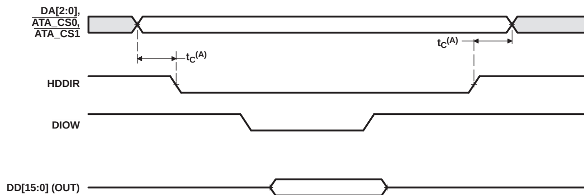
Figure 6-38. ATA/CF HDDIR Taskfile Write/Single PIO Write Timing
