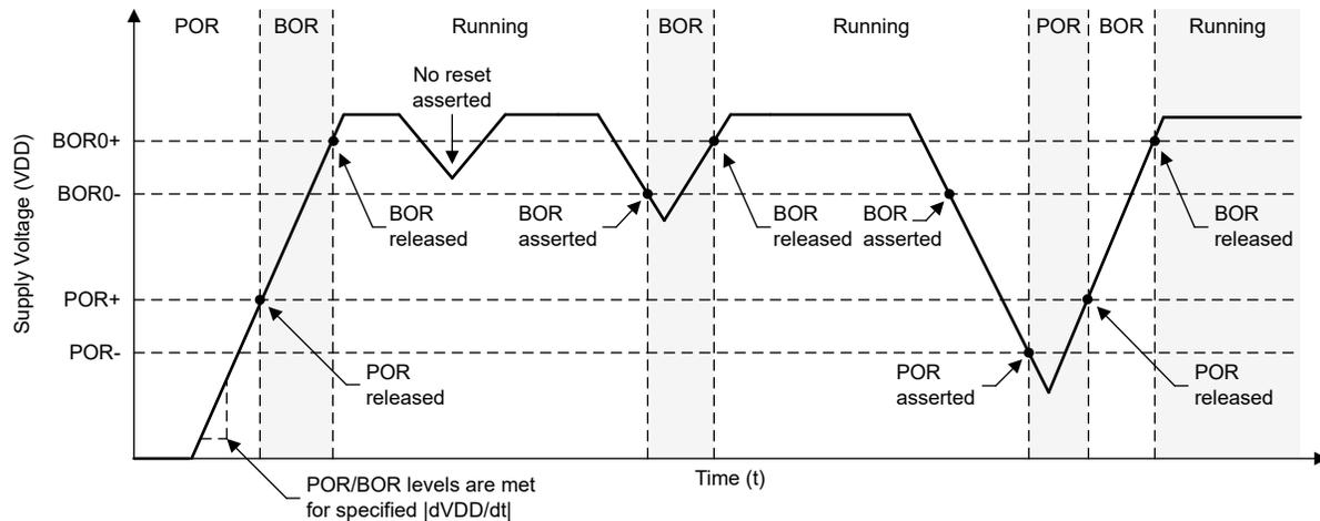
**Figure 7-1. Power Cycle POR and BOR Conditions**
