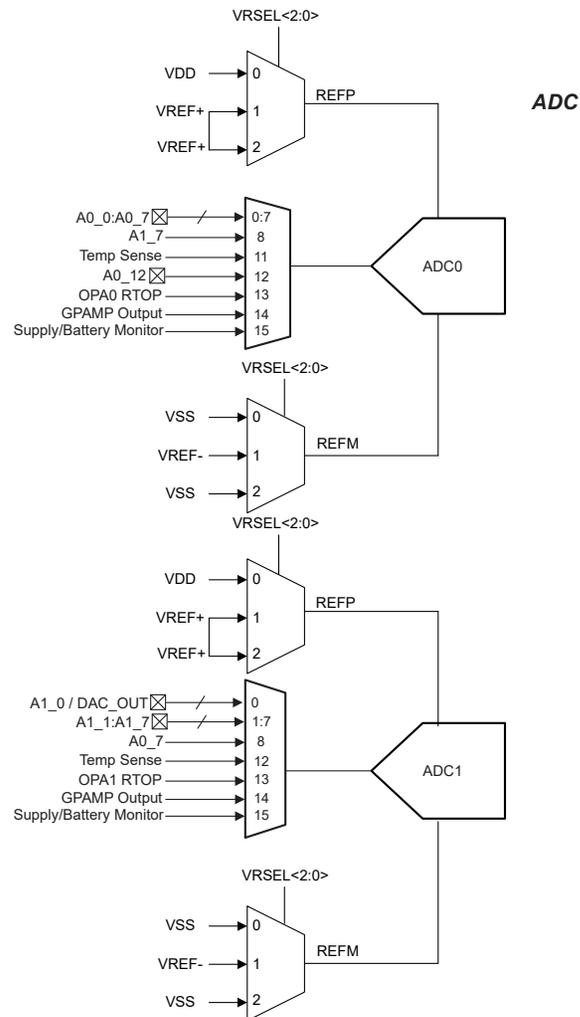
**Figure 8-3. Device Analog Connections (ADC0 and ADC1)**
