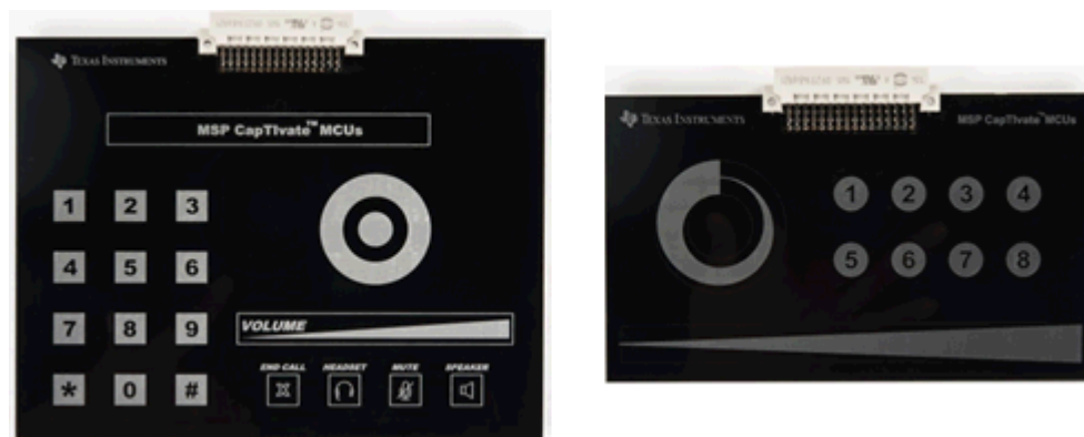
Figure 7-6. CAPTIVATE-PHONE and CAPTIVATE-BSWP Panels
