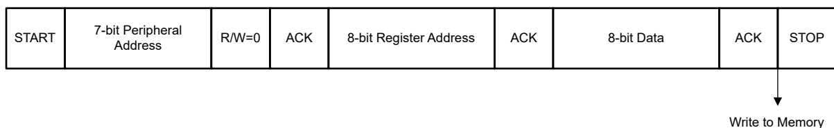
Figure 6-31. I²C Write Sequence
