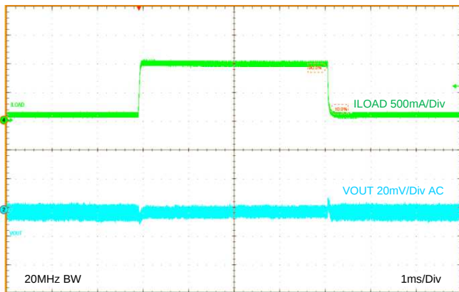
Figure 60. Load Transient V_{OUT} = 3.3\text{ V}
