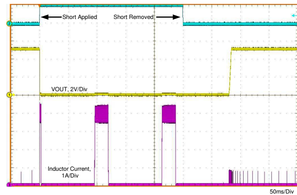
Figure 8-6. Short-Circuit Transient and Recovery
