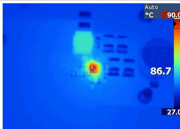
LMQ66430MC3 V_{OUT} = 3.3V 12V_{IN} , 3A, 2.2MHz Fixed
