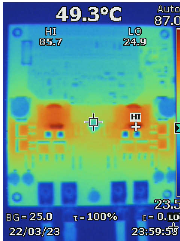
Figure 8-21. Thermal Image: Buck Mode, V_{in}=48V , V_{OUT} = 14.5V , I_{OUT}=60A , Natural Convection
