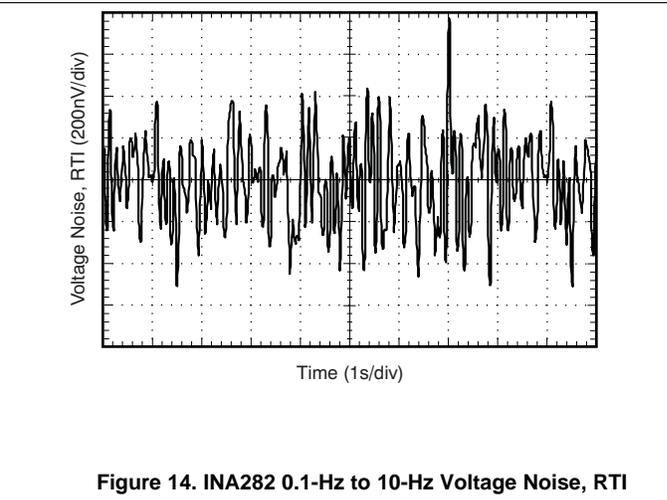
Figure 14. INA282 0.1-Hz to 10-Hz Voltage Noise, RTI
