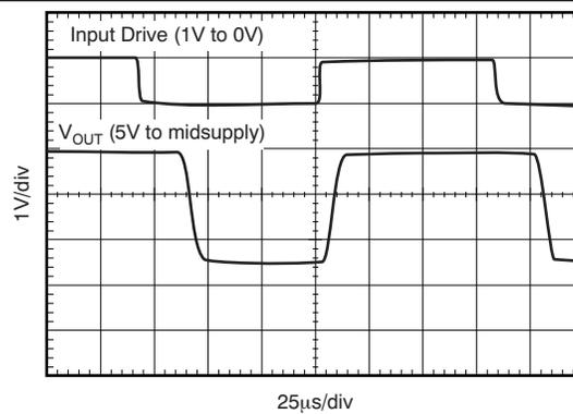
**Figure 31. Input Overload**
