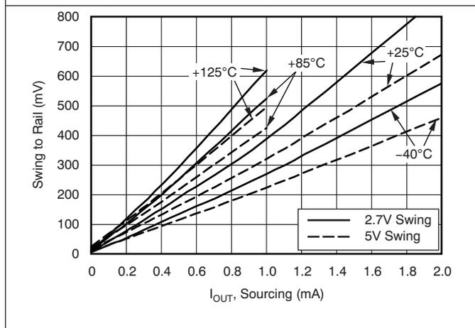
Figure 17. INA283 Swing to Rail vs Output Current
