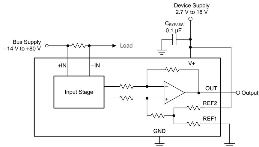
**Figure 39. Basic Connections**
