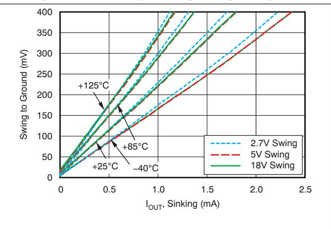
Figure 18. INA283 Swing to Ground vs Output Current
