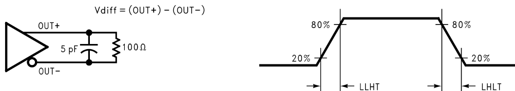
Figure 5. DS90CF563 (Transmitter) LVDS Output Load and Transition Times
