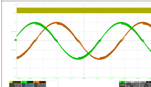
Figure 8-7. 1/256 Microstepping With smart tune Ripple Control Decay
