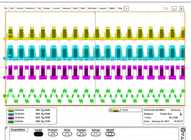
Figure 9-5. BLDC Motor Commutation 2000 RPM
