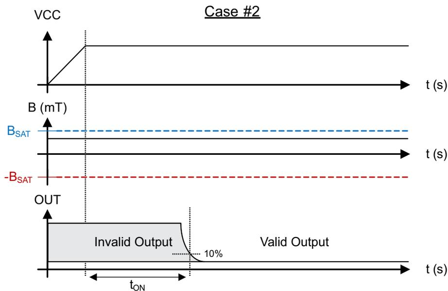
**Figure 11. Case 2: Power On When  $B > 0$ , South**
