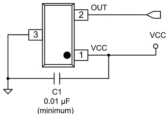
**Figure 12. Typical Application Schematic – No Filter**
