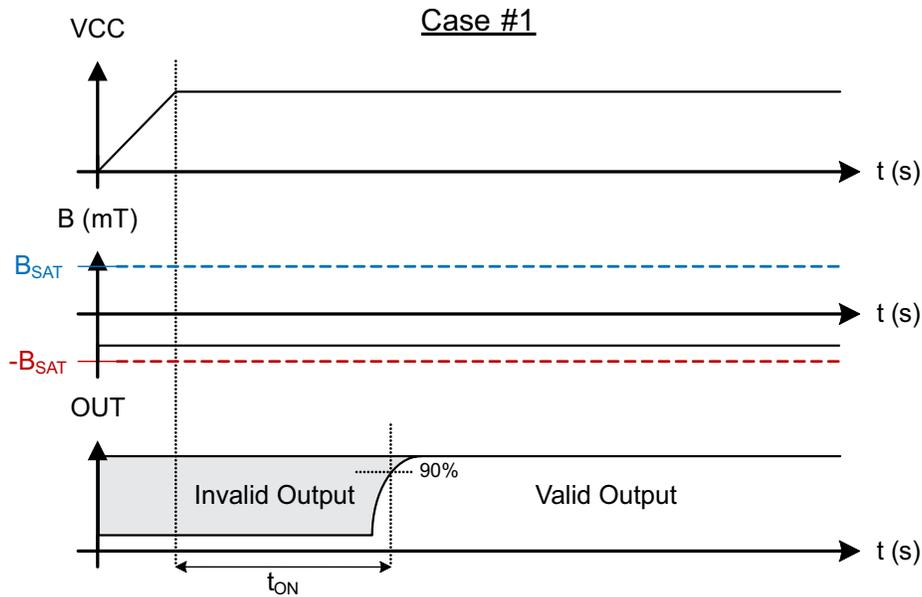
**Figure 10. Case 1: Power On When  $B < 0$ , North**
