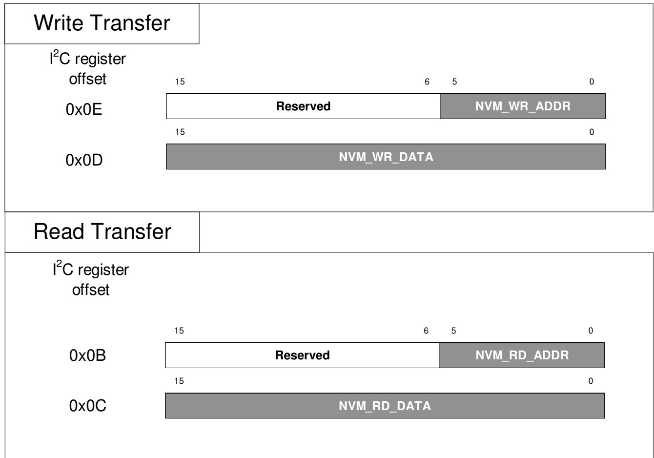
Figure 7-12. EEPROM Direct Access Using I 2 C
