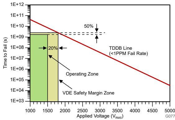
T<sub>A</sub> up to 150°C, stress-voltage frequency = 60Hz, isolation working voltage = 1500V<sub>RMS</sub>, projected operating lifetime  $\geq$ 50 years
