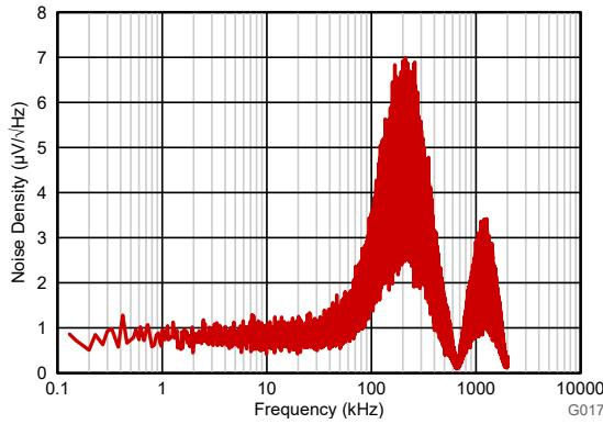
Figure 6-19. Input-Referred Noise Density vs Frequency
