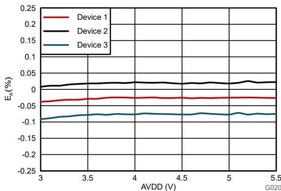
Figure 6-17. Attenuation Error vs High-Side Supply Voltage
