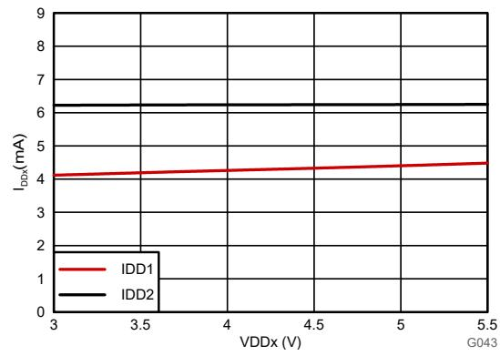
Figure 6-22. Supply Current vs Supply Voltage
