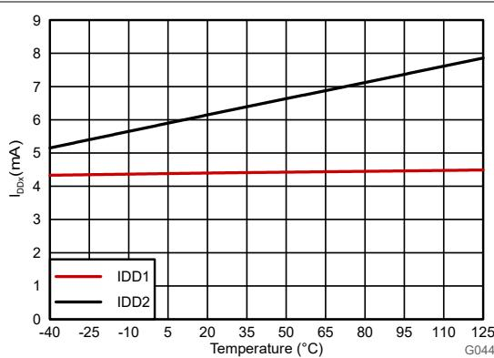
Figure 6-23. Supply Current vs Temperature
