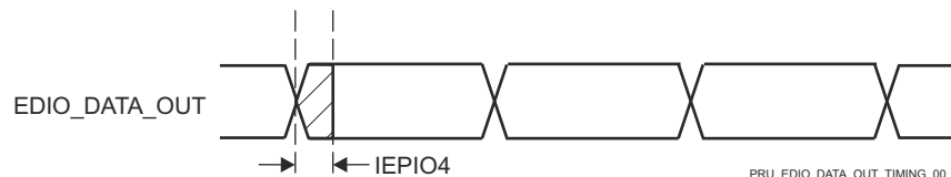
Figure 6-101. PRU_ICSSG IEP Digital IOs Timing Requirements
