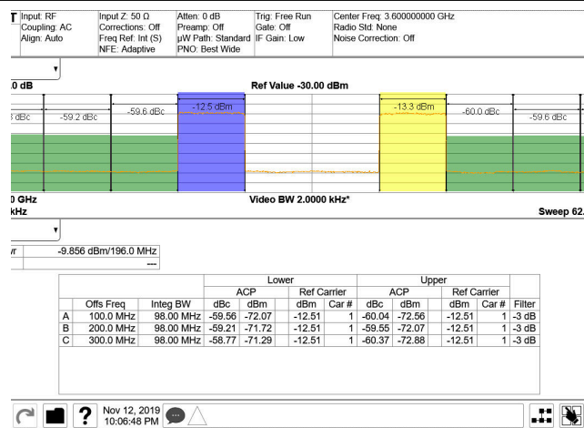
Figure 4-476. TX 20MHz LTE Output Spectrum at 3.5GHz (Band 42)
