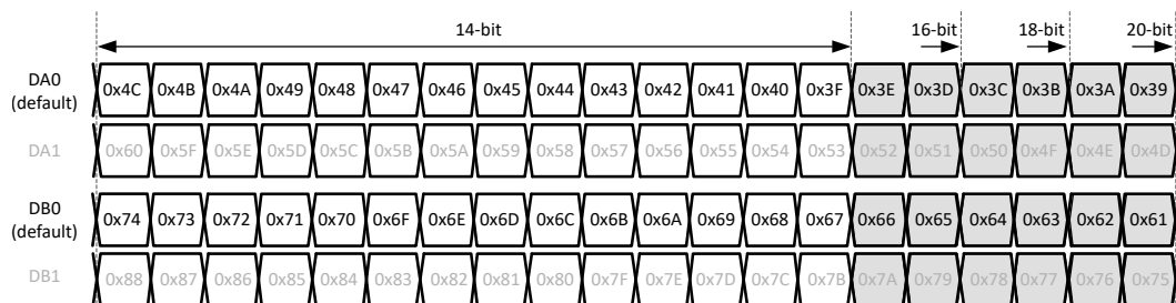
Figure 7-45. 1-wire output bit mapping
