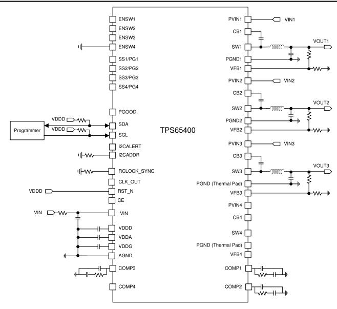
Figure 8-17. Internal Sequencing Schematic Without Host
