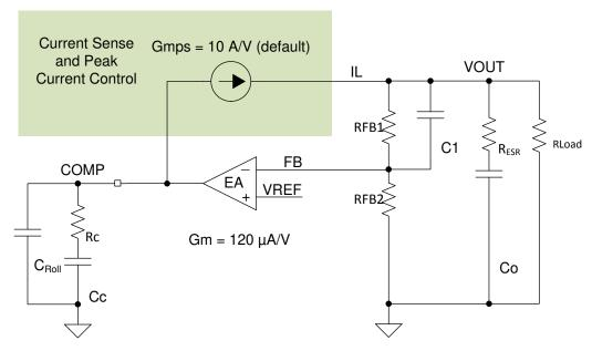
Figure 8-13. Simplified Equivalent Feedback Compensation Network
