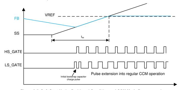
Figure 8-5. Soft-Start Under Prebiased Condition and CCM Mode Programmed
