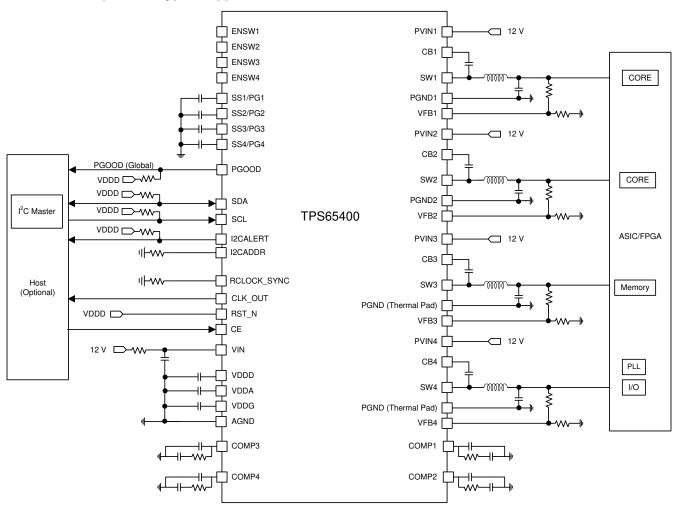
Figure 9-1. Typical Application Schematic
