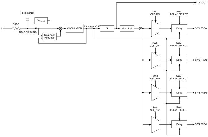
A. The frequency modulator is used for external clock synchronization.
