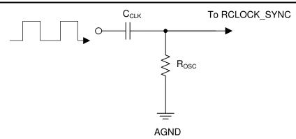
Figure 8-10. AC-Coupled Clock Synchronization
