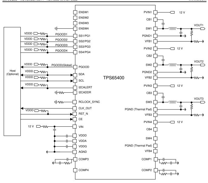
Figure 8-16. Internal Sequencing Schematic With Host
