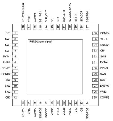
A. Thermal pad must be soldered to PCB as SW3 and SW4 power ground.
