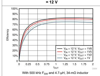
Figure 7-3. Buck3 and Buck4 Power Efficiency, VIN = 12 V
