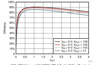
With 500 kHz and XAL6060-472 4.7- $\mu$ H, 13.2-m $\Omega$  inductor
