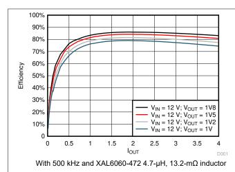
Figure 7-1. Buck1 and Buck2 Power Efficiency, VIN
