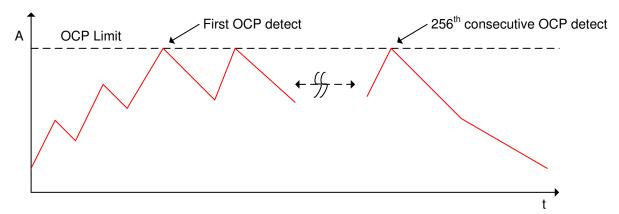
**Figure 8-11. Inductor Current During Overcurrent Event**
