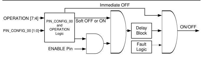
Figure 8-27. On/Off Configuration (Per Output)
