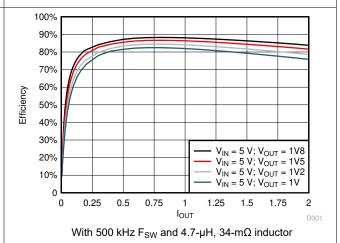
Figure 7-4. Buck3 and Buck4 Power Efficiency, VIN
