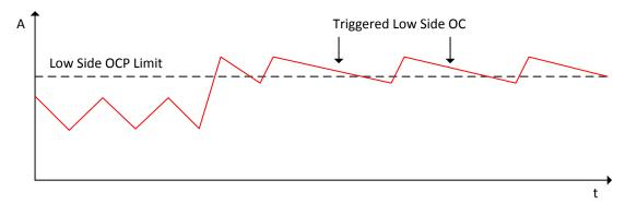
Figure 8-12. Inductor Current During Overcurrent Event With Low-Side Detection
