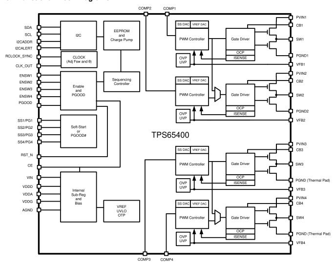
Figure 8-1. TPS65400 Functional Block Diagram
