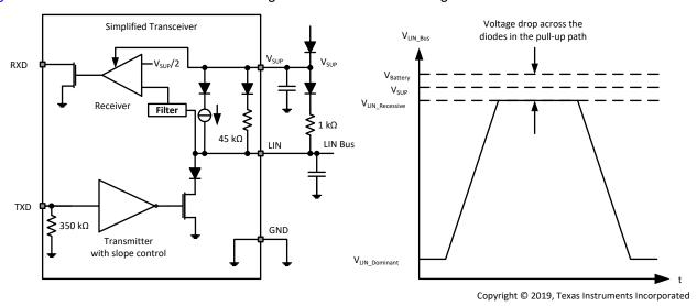
Figure 9-1. Commander Node Configuration with Voltage Levels
