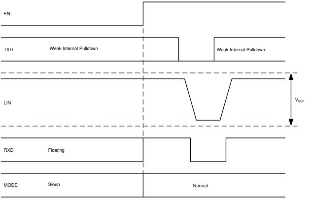
Figure 8-16. Wake-up Through EN
