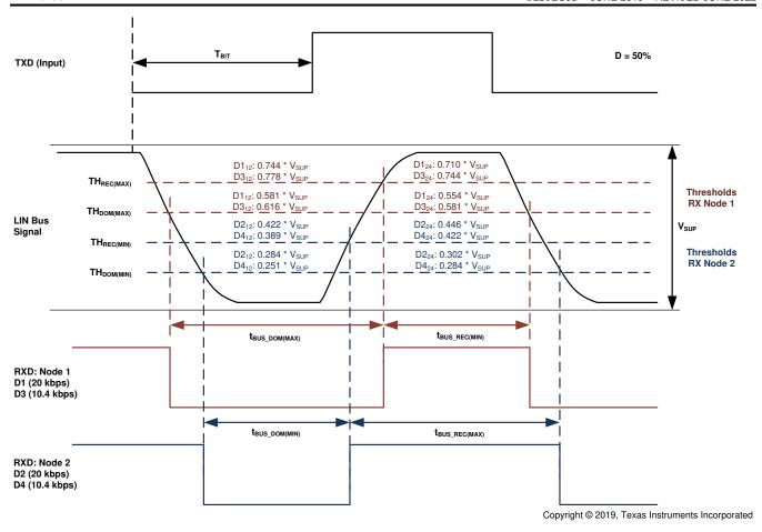
Figure 8-12. Definition of Bus Timing Parameters
