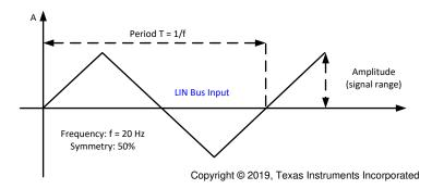
Figure 8-3. LIN Bus Input Signal
