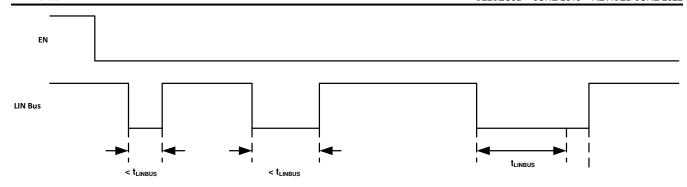
Figure 9-2. No Bus Fault: Entering Sleep Mode with Bus Recessive Condition and Wake-up
