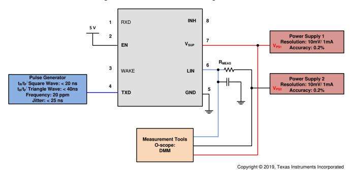
Figure 8-13. Propagation Delay Test Circuit; Param 31, 32
