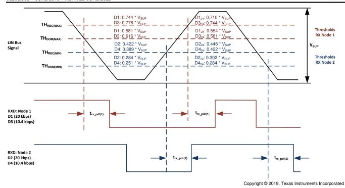
Figure 8-14. Propagation Delay
