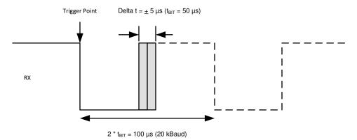
Figure 8-2. RX Response: Operating Voltage Range
