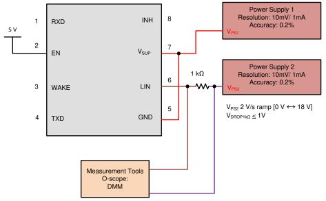
Figure 8-9. Test Circuit for I<sub>BUS\_NO\_GND</sub> Loss of GND
