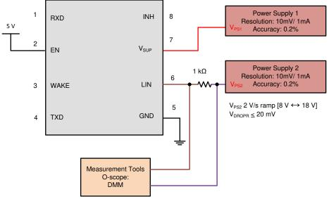
Figure 8-8. Test Circuit for  $I_{BUS\_PAS\_rec}$  Param 14
