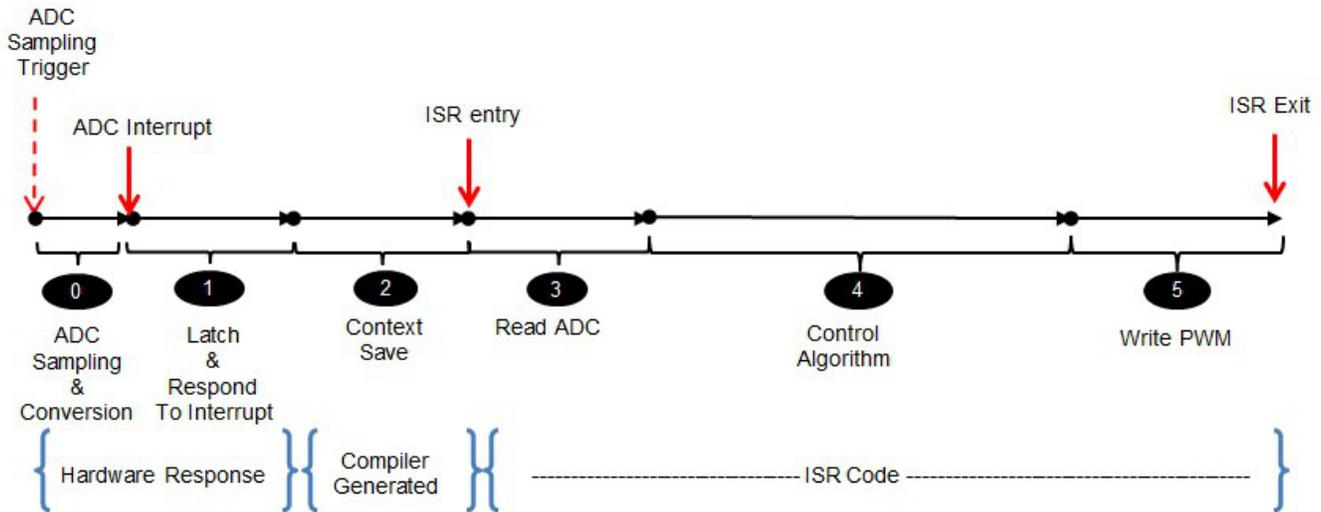
Figure 2-4. Real-Time Benchmarking Phases
