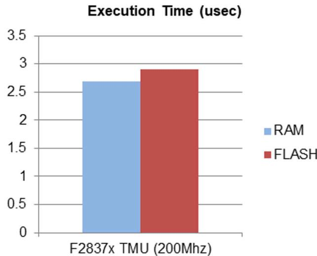
**Figure 3-7. TMS320F2837x Execution Time From RAM and Flash**
