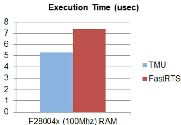
**Figure 3-4. Control Loop Execution Time Out of RAM With TMU and FastRTS**
