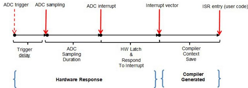
**Figure 3-1. ACI Motor Benchmark Interrupt Response Components**
