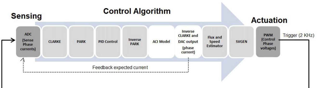
Figure 2-1. ACI Motor Benchmark Application Block Diagram
