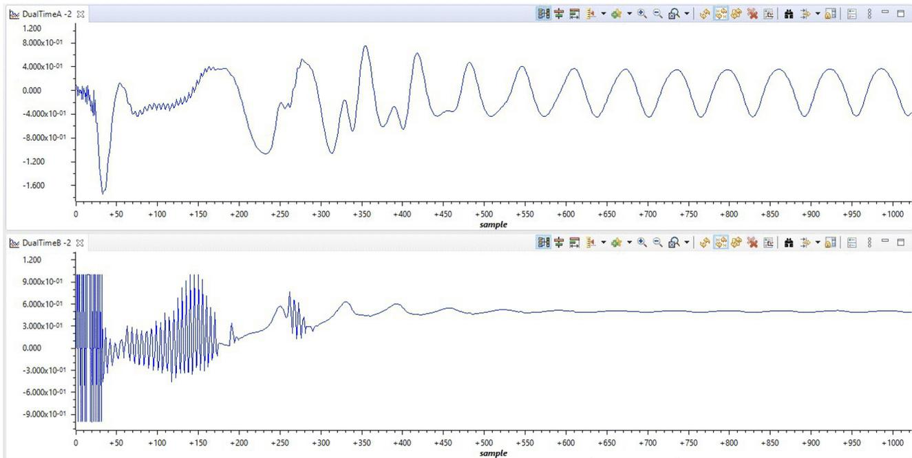
**Figure 2-2. Graphical View of Alpha Phase Current (DualTimeA) and Per Unit Motor Speed (DualTimeB)**
