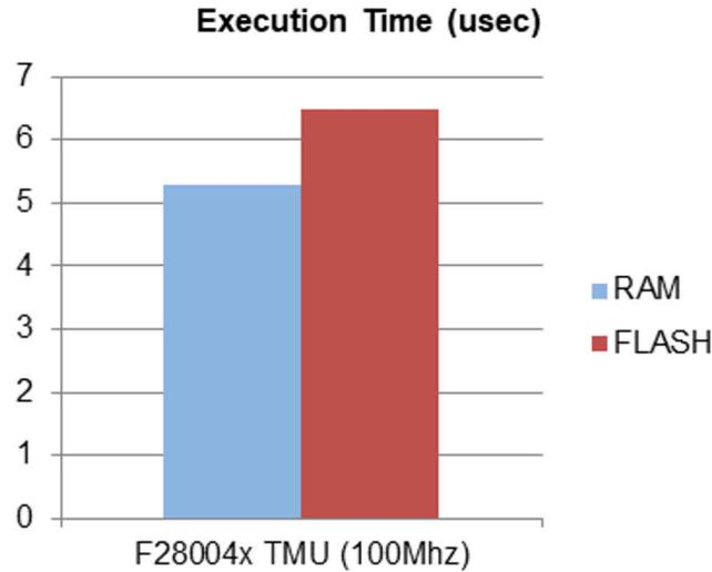
**Figure 3-6. TMS320F28004x Execution Time From RAM and Flash**
