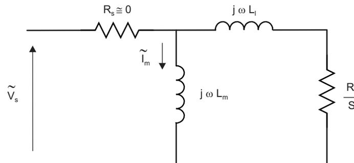
**Figure 3. Simplified Steady-State Equivalent Circuit of Induction Motor**
