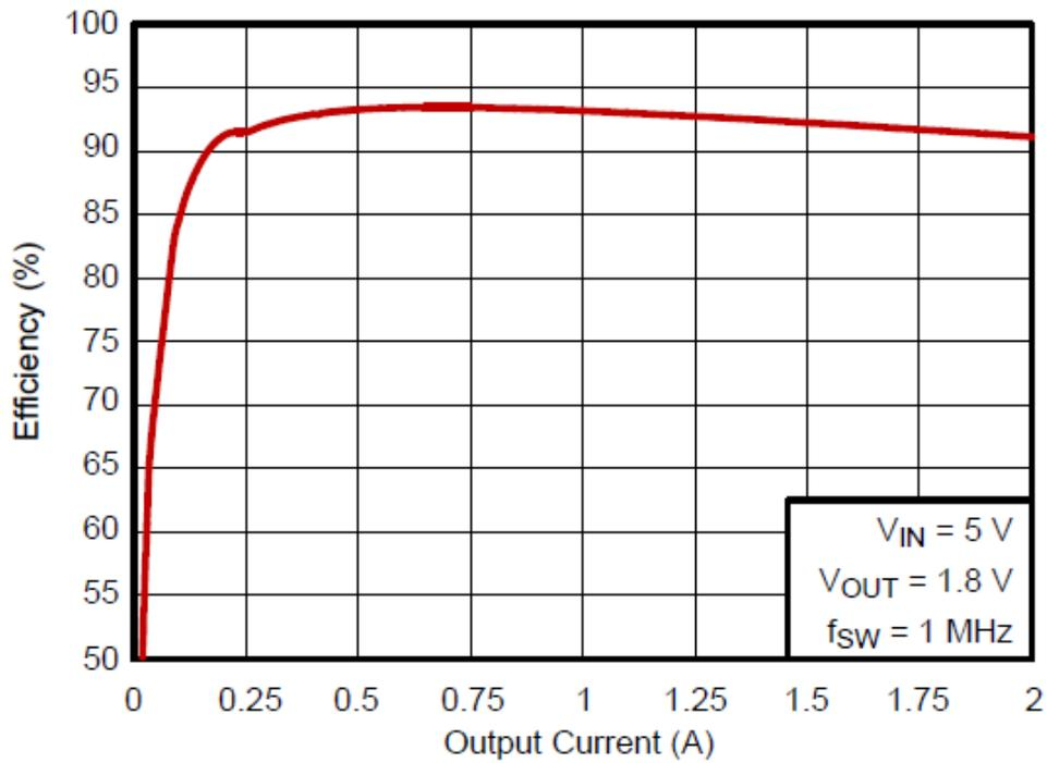
Figure 3-1. Efficiency Curve of TPS54218
