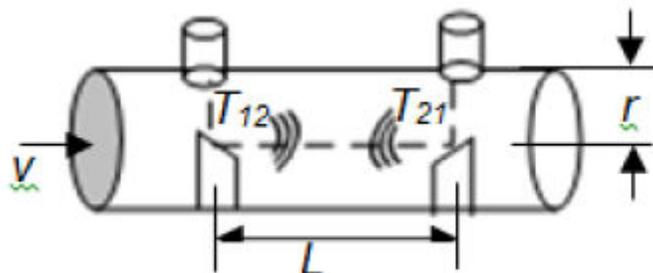
Figure 2-1. Typical Ultrasonic Water Meter
