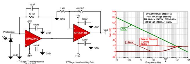
**Figure 4. Alternate Two-stage OPA140 TIA Amplifier (Stable)**
