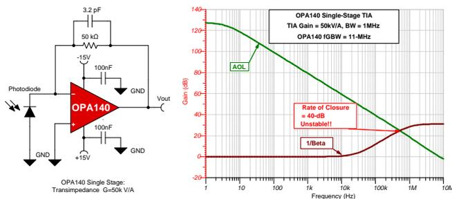
**Figure 3. Single-stage OPA140 ( $f_{GBW} = 11$ -MHz) Stability Analysis (Unstable)**
