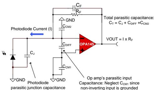
**Figure 1. Photodiode Transimpedance Amplifier**
