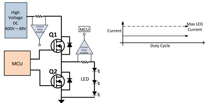
**Figure 3. Analog dimming using current sense amplifier**
