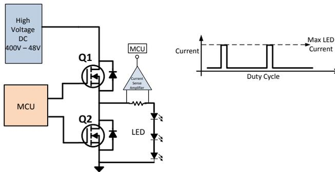
**Figure 2. PWM dimming using current sense amplifier**
