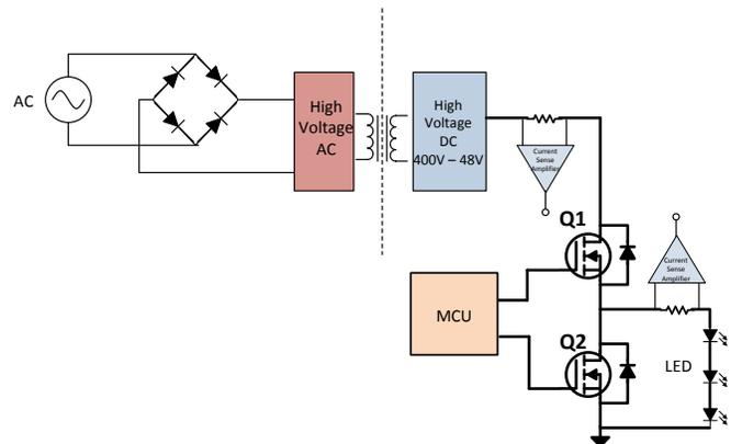
Figure 1. LED driver system control
