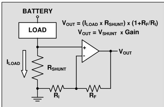
**Figure 1. Low-Side Current Sensing**
