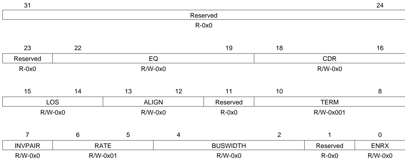
Figure 15. Receiver Configuration Register (CFGRX0/1)
