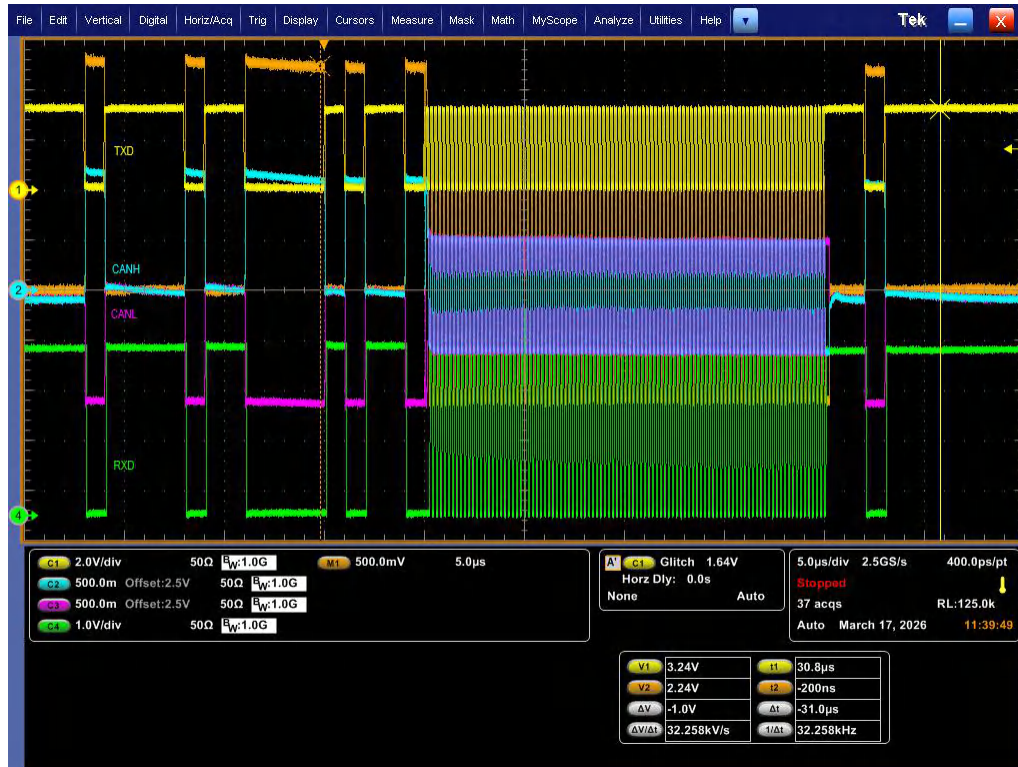
Figure 3-1. One Complete XL Frame With Arbitration
